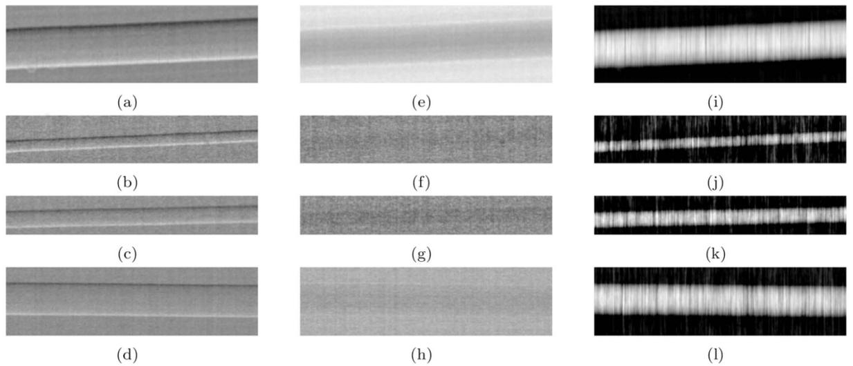
**Figure 2.** Images of the multi-wire phantom: (a–d) refraction, (e–h) attenuation and (i–l) phase. From top to bottom: sapphire 250  $\mu\text{m}$ , Nylon 100  $\mu\text{m}$ , PEEK 150  $\mu\text{m}$  and Nylon 300  $\mu\text{m}$  diameter. The vertical stripes that can be seen in panels (i–l) run parallel to the direction of integration and are a result of the presence of noise in the integrand images (a–d).
