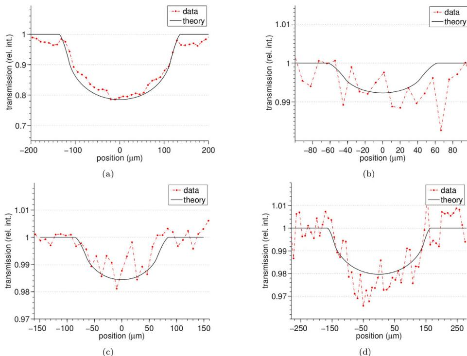
**Figure 4.** Profiles extracted from the attenuation images of the multi-wire phantom: (a) sapphire 250  $\mu\text{m}$ , (b) Nylon 100  $\mu\text{m}$ , (c) PEEK 150  $\mu\text{m}$  and (d) Nylon 300  $\mu\text{m}$  diameter.
