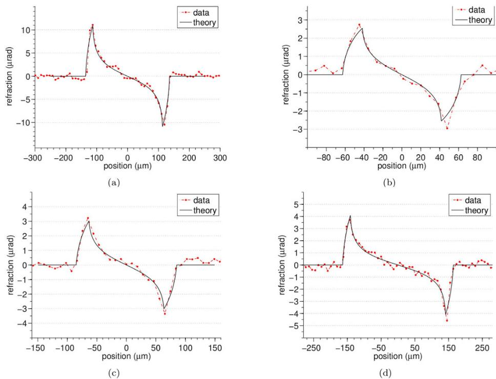
**Figure 3.** Profiles extracted from the refraction images of the multi-wire phantom: (a) sapphire 250  $\mu\text{m}$ , (b) Nylon 100  $\mu\text{m}$ , (c) PEEK 150  $\mu\text{m}$  and (d) Nylon 300  $\mu\text{m}$  diameter.
