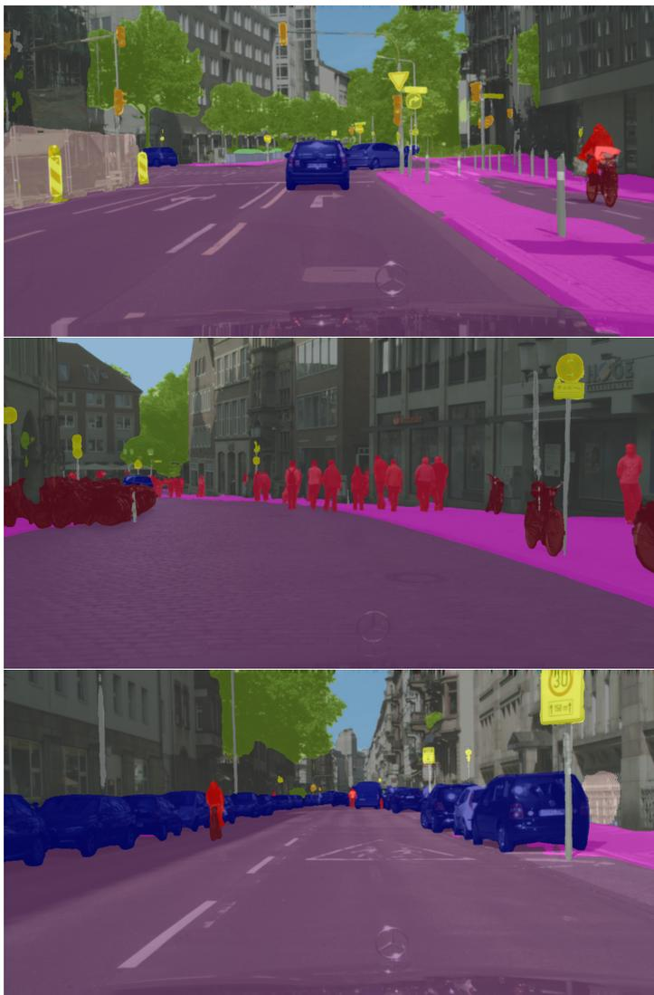
Figure 3.4: Qualitative results of the semantic segmentation task on the Cityscapes validation dataset. The CNN was trained on the Cityscapes training dataset. The corresponding color codes can be found in Figure 3.3.
