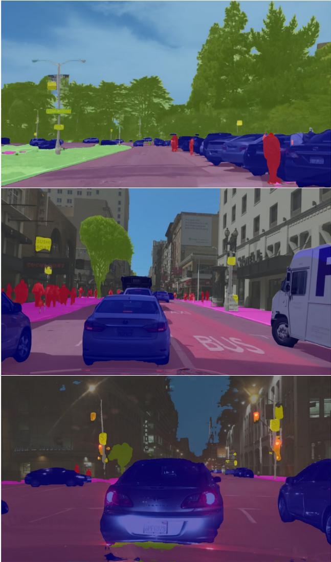
Figure 3.6: Qualitative results of the semantic segmentation task on the BDD100K validation dataset. The CNN was trained on the BDD100K training dataset. The corresponding color codes can be found in Figure 3.3.
