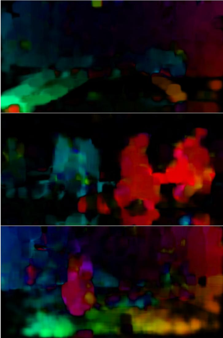
Figure 4.5: Classical optical flow estimates computed with the algorithm of Farneback [Far03]. The input images from the Cityscapes validation dataset were resized to match the size of the  $P_2$  feature maps. The direction of movement in the image plane is encoded in the hue of the color, while the magnitude is encoded in its brightness.
