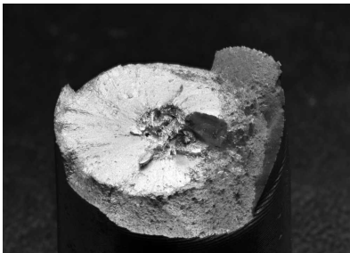
Upper Fracture Surface
