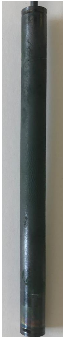
MC-5: 1200 °C during 15 min
