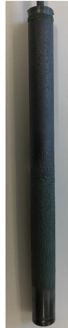
MC-6: 1350 °C during 5 min
