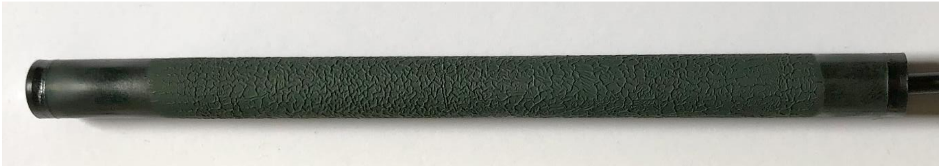
sample MCs-2: transient with 8 K/s, then 1400 °C during 240 s
