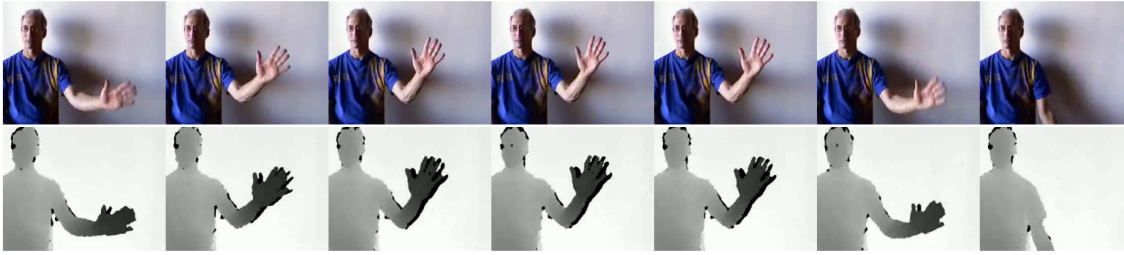
Figure 14: Example of a gesture in the multimodal IsoGD dataset. The data captured by a color-based camera is strongly influenced by the illumination conditions e.g. the shadows produced by the light source to the left. However, the depth data can have problems recognizing even the hand if the hand has the same depth as other objects close to it e.g. the hand touching the wall.
