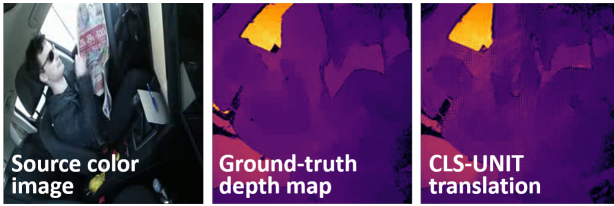
Figure 54: Color-to-depth translation. Source color image, ground-truth depth map (estimated with a Kinect) and the CLS-UNIT translation result.
