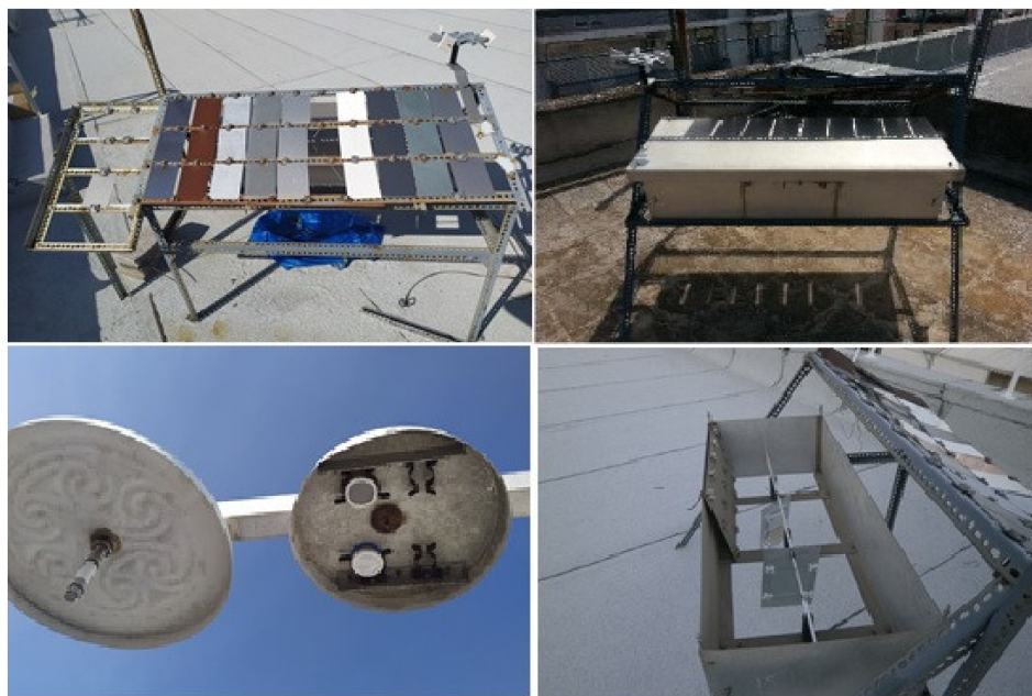
Figure 1. Views of the ACAS exposure site equipped with a metal rack on the roof of a building located in the Athens center, facing south. The rack consists of an inclined plane, for displaying samples of material under unsheltered conditions, and an aluminum box with an open bottom, for the exposure of materials' specimens under sheltered conditions. In addition, there is a mast with an arm that holds two rain shields, in the form of discs, under which passive particle collectors and diffusive samplers for gaseous pollutants are exposed [80,81].
