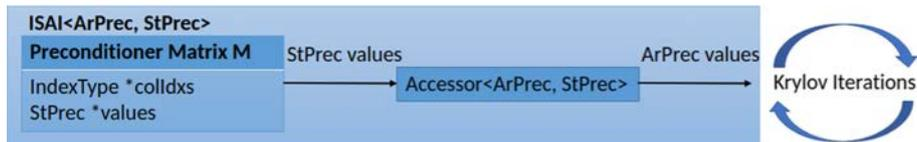
**Fig. 3.** The *memory accessor* converts STPREC values to ARPREC on the fly, reducing memory movement.
