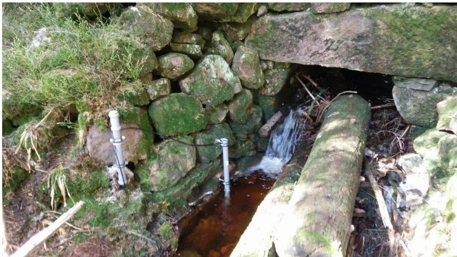
Figure C.4: Position of the probe installed at the starting point of the Schönmünz stream at the outlet of the Wildsee (WA).
