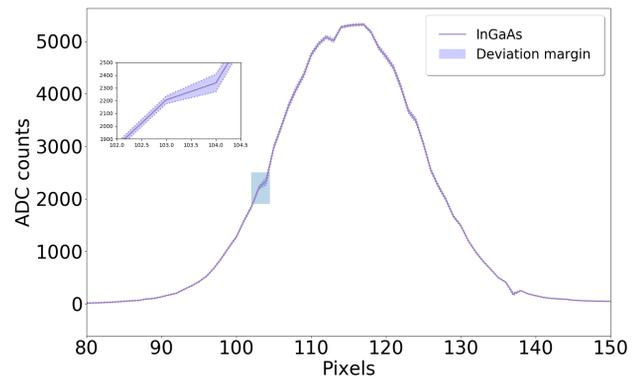
Figure 6: Single-shot laser beam profile of 1560 nm laser.
