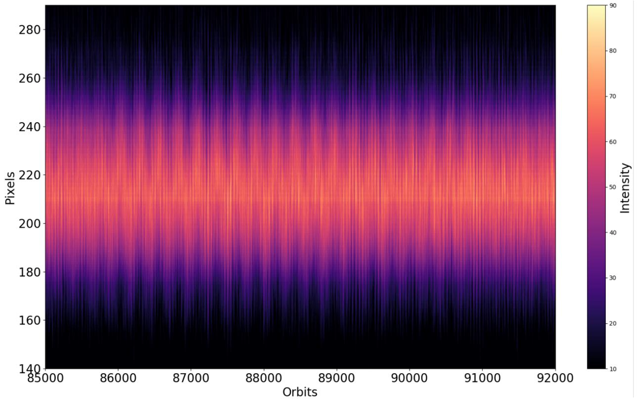
Figure 4: Evolution of the profile measured by KALYPSO: the total orbits recorded were  $10^5$  and cut short for better visualization.
