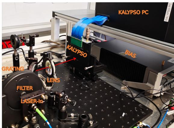
Figure 2: Grating spectrometer with DAQ of the EOSD setup.
