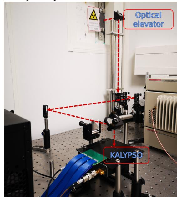
Figure 3: Optical setup for energy-spread measurement at the VLD port.
