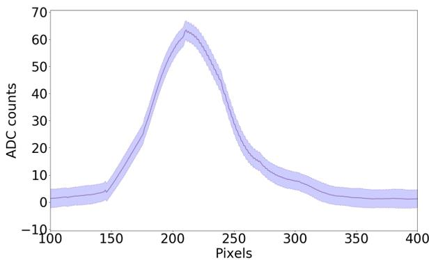
Figure 5: Single-turn profile of the incoherent synchrotron radiation measured by KALYPSO.
