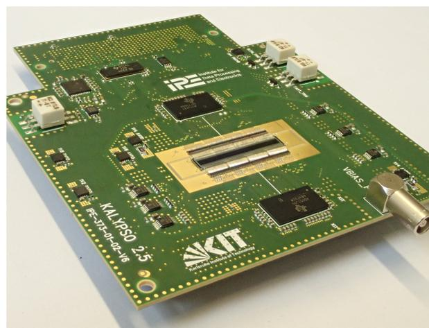
Figure 1: A fully assembled KALYPSO board with Si sensor and optimized sensitivity towards visible light.
