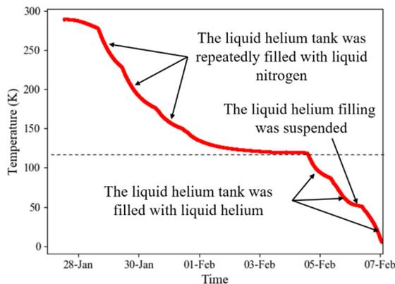
Figure 3: TGU temperature during the cool-down process.
