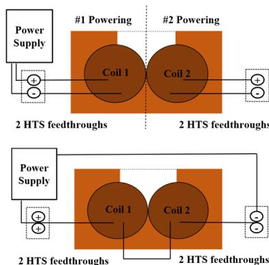
Figure 7: Diagram to explain the magnet powering test conditions for (above) this step and (below) the upcoming experiments.
