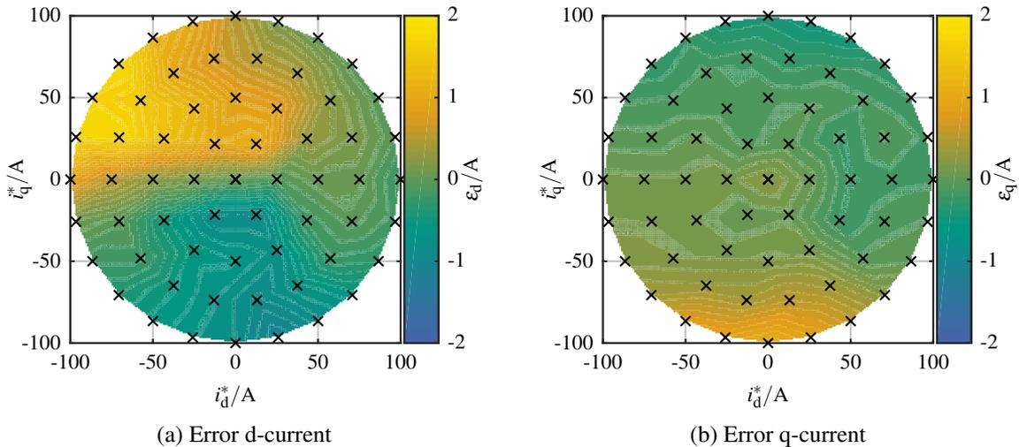
Fig. 5: Difference between the currents of the PHIL inverter test bench and the machine measured in the dq-current-plane with  $i_d^*$  and  $i_q^*$  as setpoint values at  $1000 \text{ min}^{-1}$
