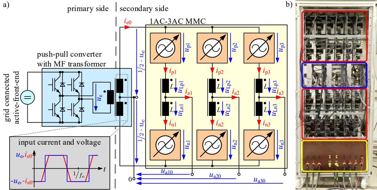
Fig. 4: Overview of the PHIL test bench
