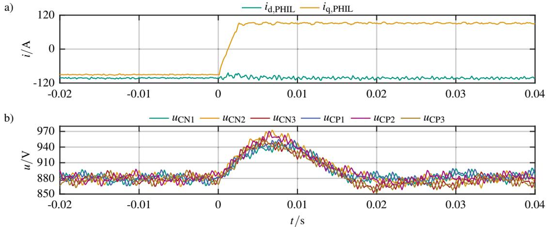
Fig. 8: Arm capacitor voltages of the SPMMC during torque reversal step from  $-70\text{ Nm}$  to  $+70\text{ Nm}$  at  $+4000\text{ min}^{-1}$
