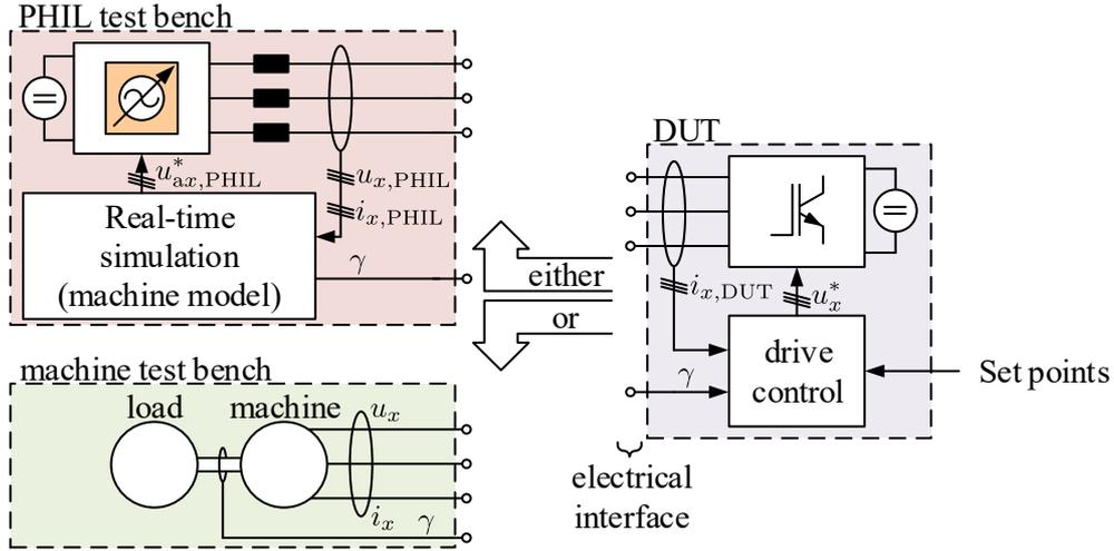
Fig. 1: Overview of testing the device under test either with a PHIL test bench or with a machine test bench
