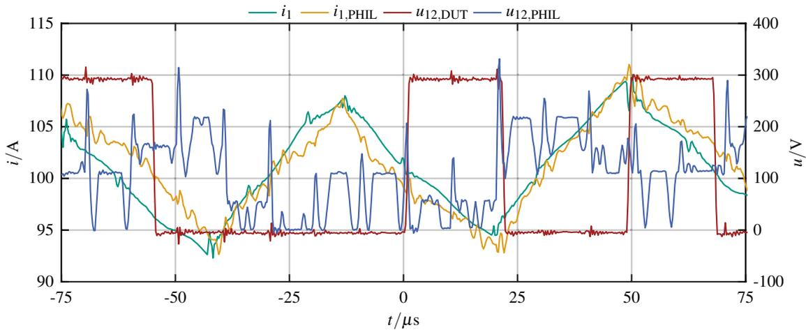
Fig. 6: Scope measurement of machine current  $i_1$  and emulated current of the PHIL  $i_{1,\text{PHIL}}$  in the same operating point
