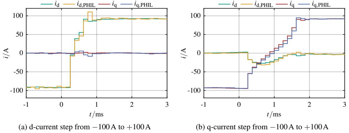
Fig. 7: Current reversal step in either d- or q-current in comparison with the machine and PHIL test bench at  $1000\text{ min}^{-1}$
