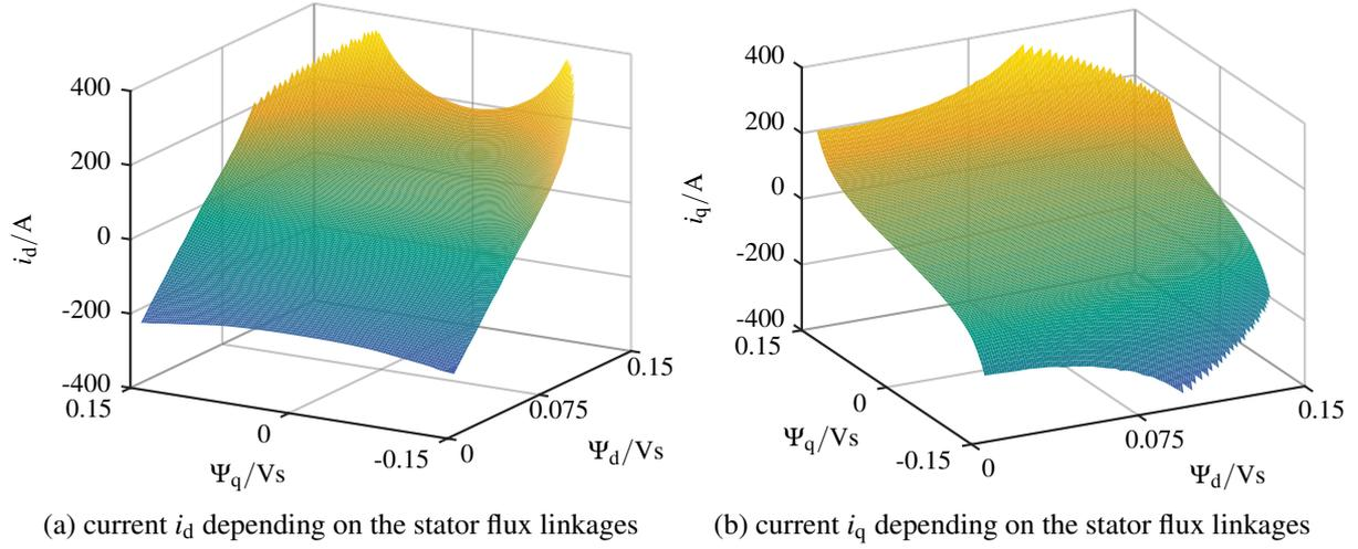
Fig. 3: stator currents depending on the stator flux linkages  $\Psi_d$  and  $\Psi_q$
