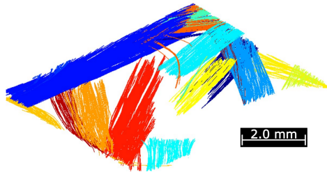
Figure 6.12: Close-up of the tracked and clustered fiber bundles within the marked region in Figure 6.11 (b) (figure by Schöttl et al. [242]*).
