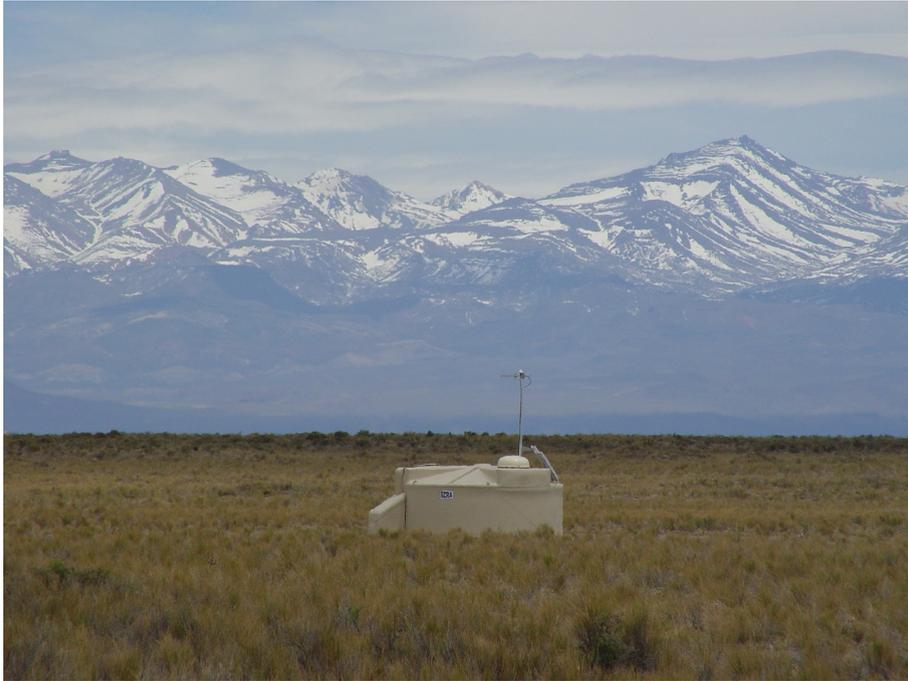
**Figure 4.2.:** Image of a surface detector. Visible is the battery box on the left, antennas on top and the solar panel on the right side of the tank. In the background the Argentinian Andes can be seen. From [33]
