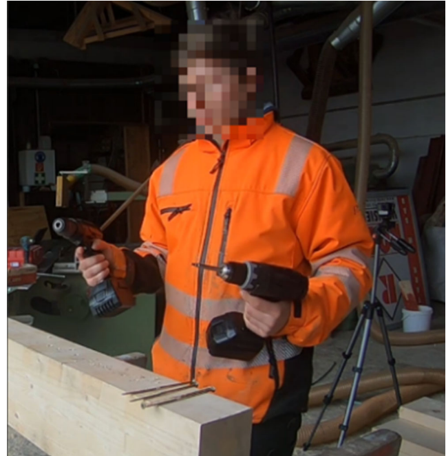
Fig. 5 Comparison of two blackened cordless screwdrivers for an objective evaluation of technical usability aspects by a professional worker
