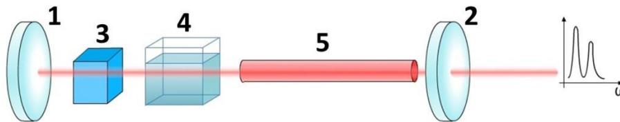
**Fig. 1.** 1, 2 mirrors 3 – passive q-switch, 4 - SLFRS active sample 5 –ruby crystal
