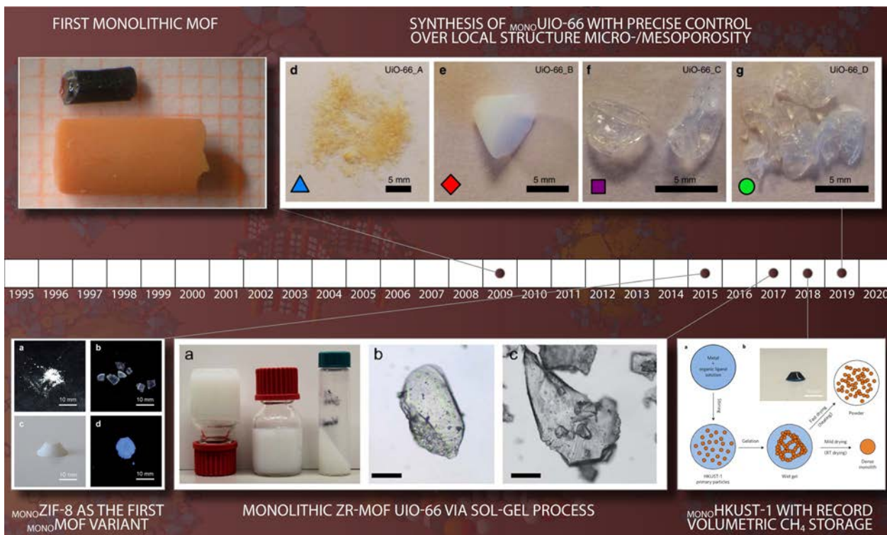
Figure 12. Illustrative timeline of the milestones in monolithic reticular materials. First monolithic MOF (reproduced with permission from ref. [291], Copyright 2009 The Royal Society of Chemistry). MONOZIF 8 as the first MONOMOF variant (reproduced with permission from ref. [292], Copyright 2015 The Royal Society of Chemistry). Monolithic Zr MOF UiO 66 via sol gel process (reproduced with permission from ref. [293], Copyright 2017 The Royal Society of Chemistry). MONOHKUST 1 with record volumetric \text{CH}_4 storage (reproduced with permission from ref. [294], Copyright 2018 Springer Nature). Synthesis of MONOUiO 66 with precise control over local structure and micro /mesoporosity. (reproduced with permission from ref. [295], Copyright Springer Nature 2019).
