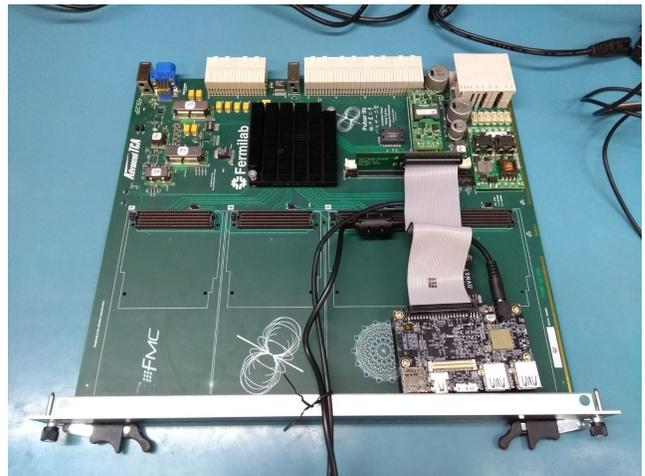
Fig. 5. Development setup with the Ultra96 sitting on top of the Pulsar-2b.
