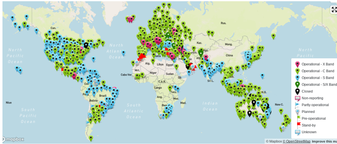
Fig. 2.8.: Mapping distribution of the S-, C- and X-band country-level weather radar network by countries, screenshot from the World Meteorological Organization (WMO) radar database website ( wrdb.mgm.gov.tr )
