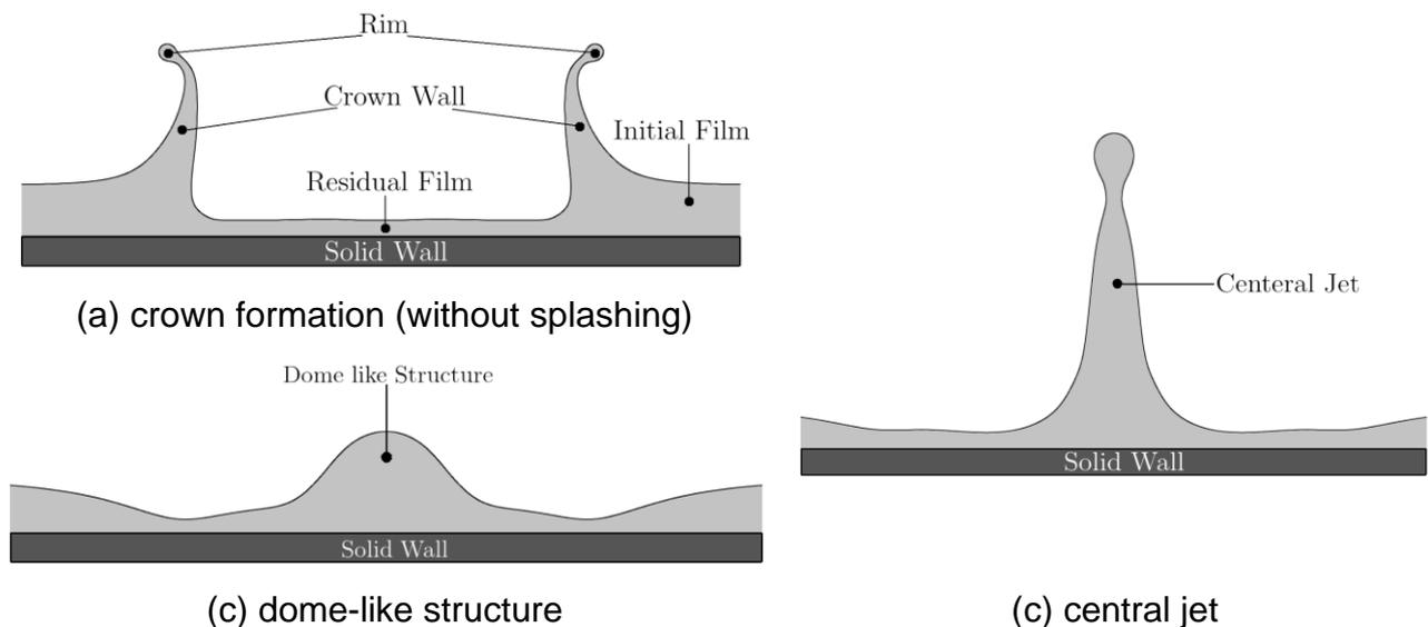
Fig. 1: Different outcomes of drop impact on a liquid film
