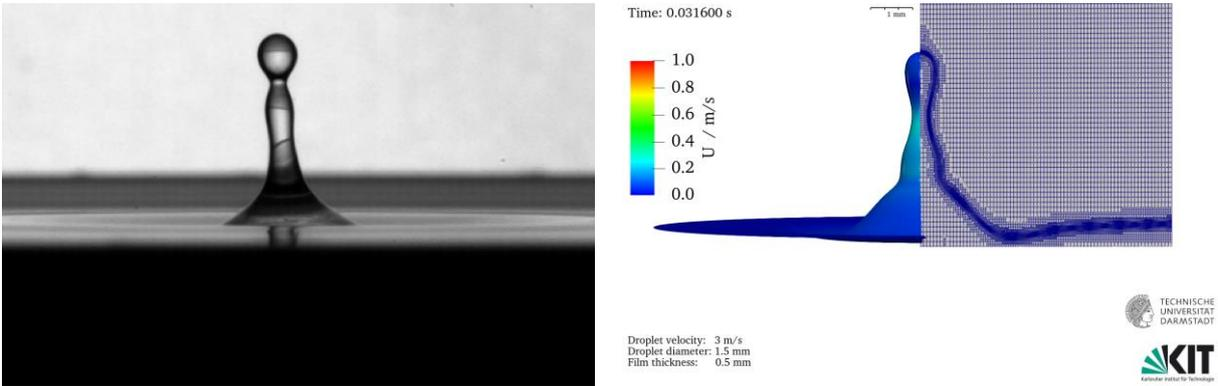
Fig. 2: Comparison between experimental and numerical simulation
