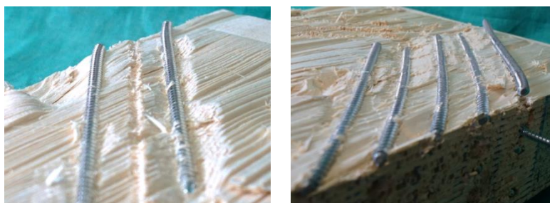
Figure 19. Plastic deformation of screws 6x200 (left) and 8x300 (right).
