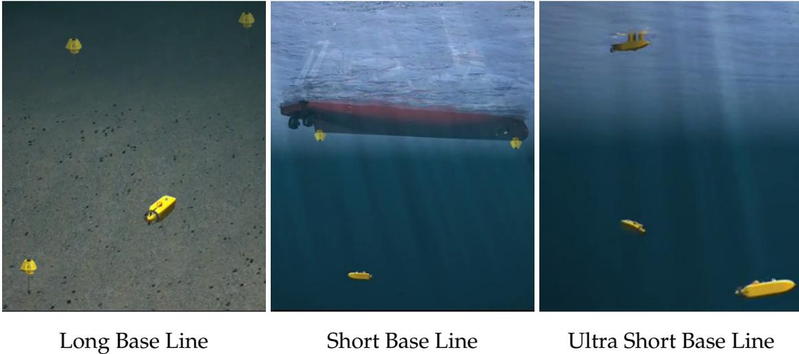
Figure 2.4.: Illustration of acoustic localization systems divided by the base line they use.
