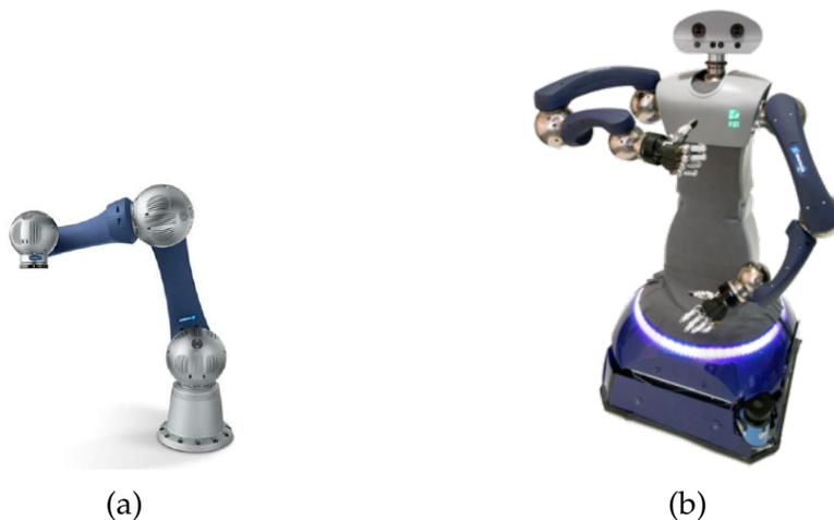
Figure 4.2.: Robots used for the arm experiments. (a) Robotic arm Schunk Powerball Lightweight Arm LWA 4P (Memar et al. [157]) (b) Humanoid robot HoLLiE (FZI [105]).
