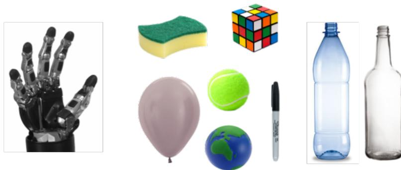
Figure 5.26.: Soft-grasping problem definition. Given a limited number of hand primitives, adapt them to grasp objects with different shapes, stiffness and sizes without knowing their exact geometric and physical properties. Use compliant control without force sensors to control a real anthropomorphic robot hand.
