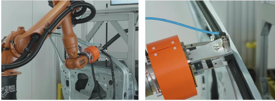
Figure 5.20.: Mounting of flexible polymer sealing strips to car doors with active compliance control. Application of the winning team FLAI<sup>2</sup>R during the European Robotics Challenges (EuRoC) [220].
