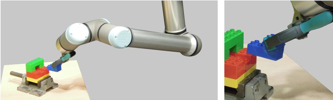
Figure 5.23.: Setup for the toy assembly with the UR10e robot. *Left*: The passive object is clamped in a vice and glued to a surface with adhesive tape. *Right*: A non-actuated gripper holds the active object in place with glued jaws. The elasticity of the material adds uncertainty to the system.
