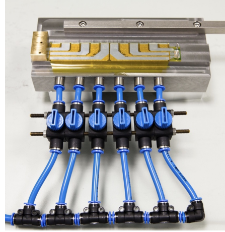
(b) Ladder after gluing the HDI to six chips on the vacuum chuck [5].
