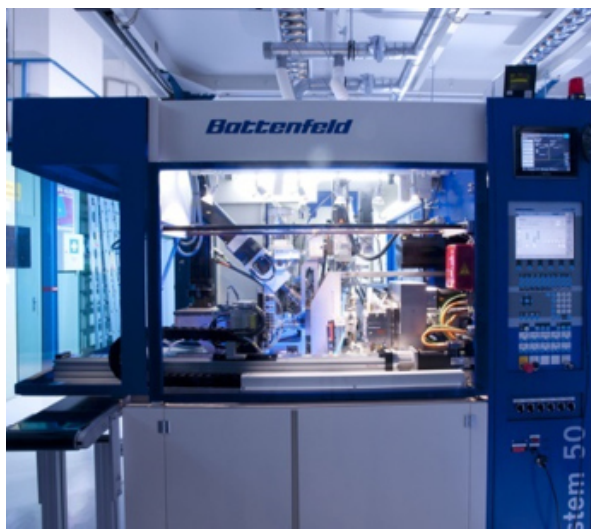
Figure 1: The Battenfeld Microsystem 50 injection molding machine used for replication of the artificial swarf samples.
