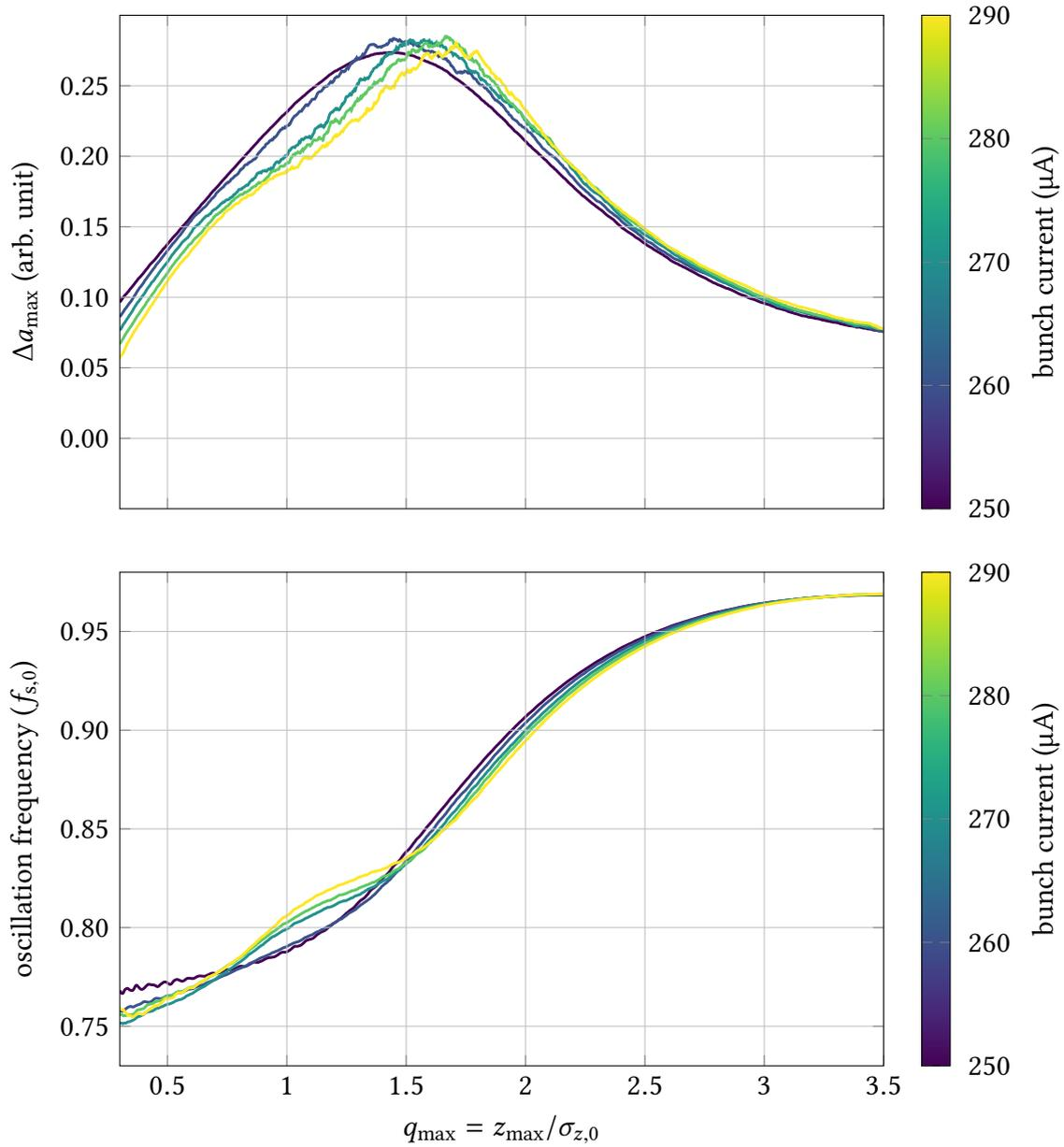
Figure 5.8.: Shown are the amplitude difference (top) and oscillation frequency (bottom) of particles trajectories for the bunch currents  $I = (250, 260, 270, 280, 290) \mu\text{A}$ . As the data scatters a lot, only a moving average over  $q_{\max}$  is displayed to enable a comparison between different currents.
