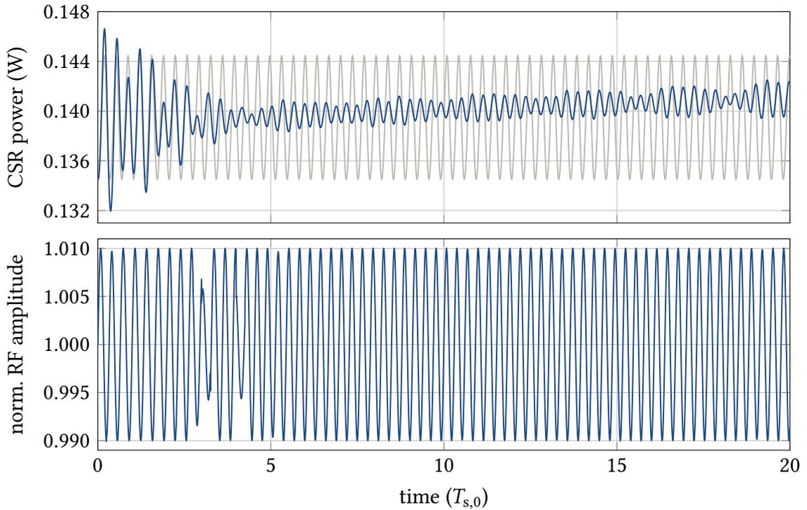
Figure 7.25.: Mitigation of the oscillations in the emitted CSR power (top) and the underlying micro-bunching dynamics by a PPO agent trained on the feature vector derived from the CSR power signal. The modulation of the RF amplitude chosen by the agent (bottom), is almost always at the maximum amplitude. Dynamic adjustments to the changing micro-bunching dynamics are made almost exclusively via the modulation frequency as shown in Fig. 7.27.
