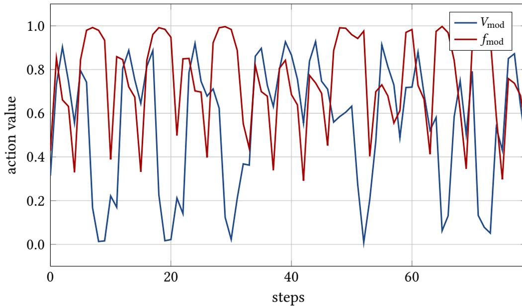
Figure 7.16.: Actions chosen by the PPO agent for the sequence displayed in Fig. 7.14. Both, the amplitude and the frequency of the modulation are dynamically adjusted by the RL agent to mitigate the micro-bunching dynamics.
