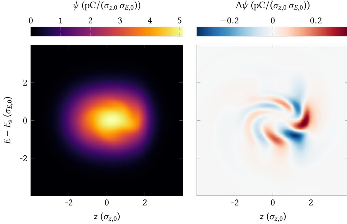
Figure 3.8.: Snapshot of the charge distribution in phase space in the regular bursting regime (left). The deformations of the distribution are emphasized by the subtraction of the temporal average, revealing a characteristic pattern of micro-structures (right).
