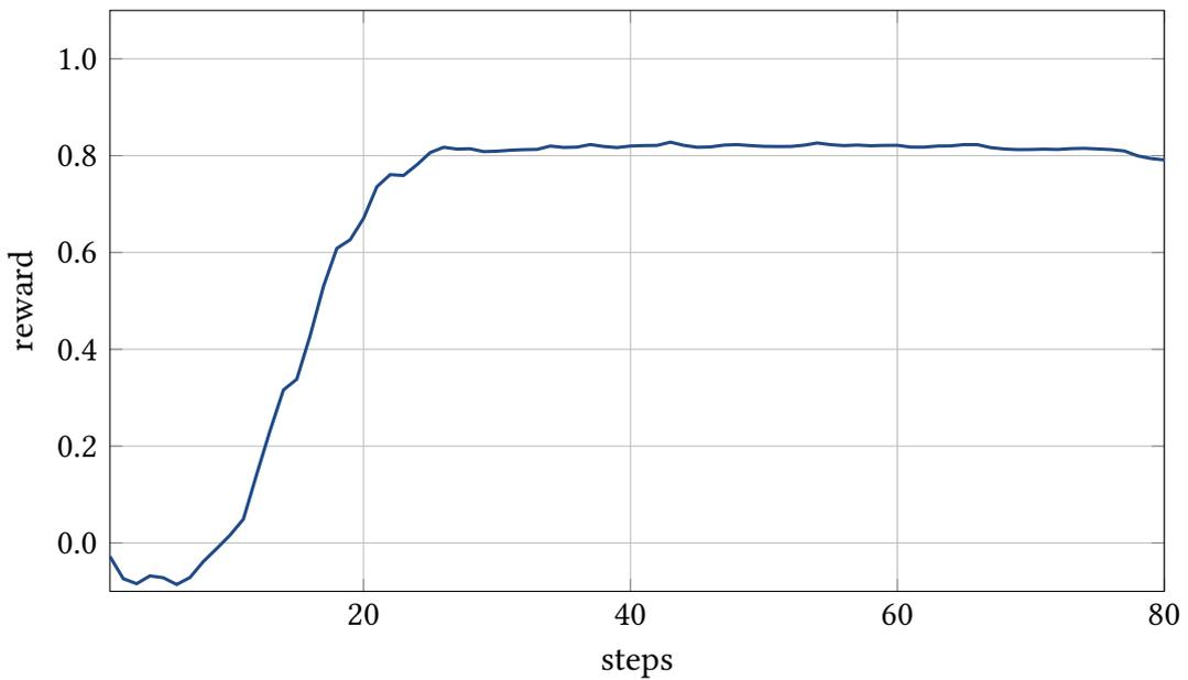
Figure 7.28.: Sequence of rewards corresponding to the mitigation of the micro-bunching dynamics shown Fig. 7.25. The obtained reward quickly reaches and stabilizes at values around  $R_t = 0.8$ , which allows the agent to achieve the highest return yet,  $G_0 = 52.18$ .
