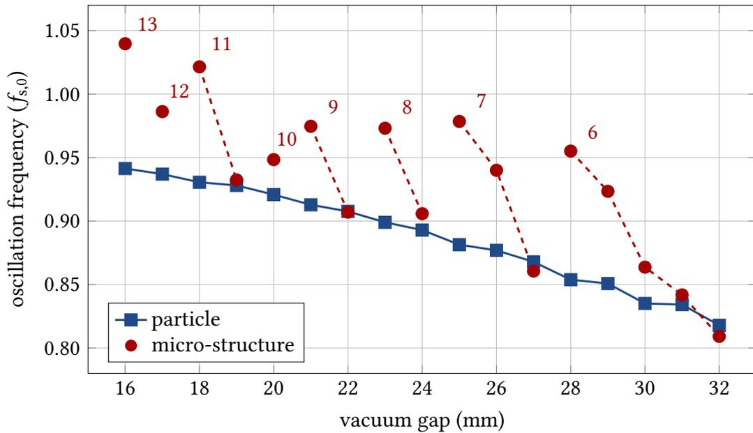
Figure 5.11.: Modifying the CSR shielding by varying the vacuum gap leads to altered micro-bunching dynamics in the longitudinal phase space. While the single particle frequency at the micro-structure position (blue squares) increases smoothly with reduced vacuum gap, the oscillation frequency of the micro-structures themselves (red circles) grows much faster and shows an abrupt change when an additional structure is observed.
