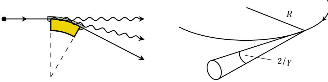
(a) Emission of synchrotron radiation in a bending magnet
