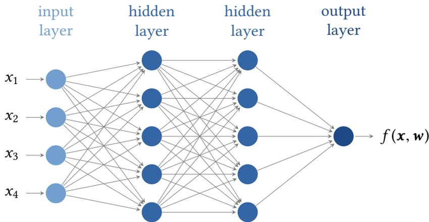
Figure 4.4.: A simple example of a feedforward neural network. The four-dimensional input vector  $\mathbf{x}$  is processed by two hidden layers with five nodes each, before a single output node computes the output  $f(\mathbf{x}, \mathbf{w})$ .
