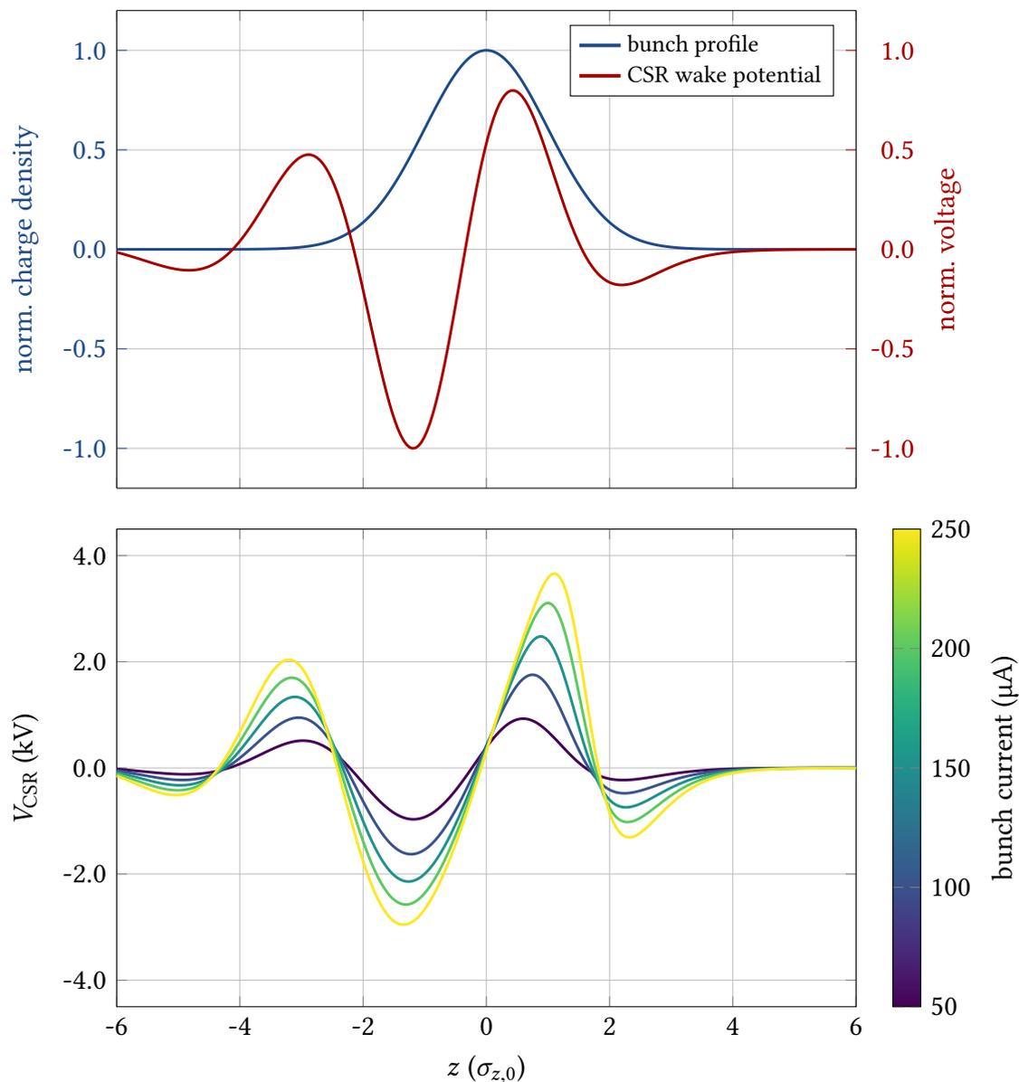
Figure 5.2.: CSR wake potential for a Gaussian bunch profile (red and blue, top) and for the bunch currents  $I = (50, 100, 150, 200, 250) \mu\text{A}$  below the instability threshold of  $I_{\text{th}} = 260 \mu\text{A}$  (bottom). Shown are the respective temporal averages for simulations (including damping and diffusion) of the parameter settings defined for  $\mathcal{D}_2$  in appendix A.1 (with  $g = 32 \text{ mm}$ ).
