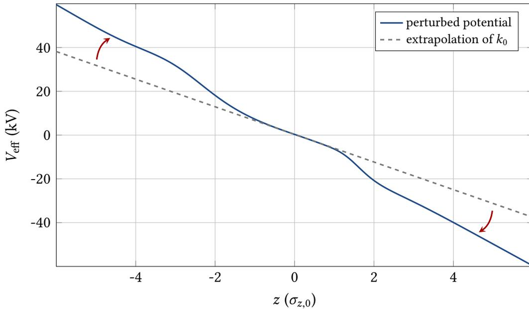
Figure 5.13.: The dynamic perturbation of the slope of the effective potential at the synchronous position  $k_0$  is found to be critical for the micro-structure formation process. By modulating the RF amplitude, the CSR-induced perturbation can be partially counteracted.
