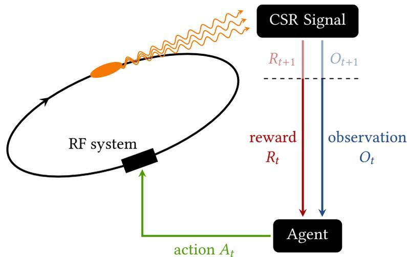
Figure 6.1.: General feedback scheme for the implementation of RL-based micro-bunching control at KARA. The agent receives an observation  $O_t$  and reward  $R_t$  calculated based on the measured CSR power signal  $P_{\text{CSR}}(t_i)$  and chooses an action  $A_t$  that defines the RF amplitude modulation for the subsequent time step.
