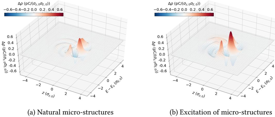
Figure 7.3.: (a) The naturally occurring micro-bunching dynamics lead to the formation of distinct micro-structures in the longitudinal phase space. (b) An RF amplitude modulation at the micro-structure frequency,  $f_{\text{mod}} = f_{\text{ms}}$ , and with  $V_{\text{mod}} = 0.05 V_0$ , leads to an amplification of the already naturally occurring structures by nearly 50 percent.
