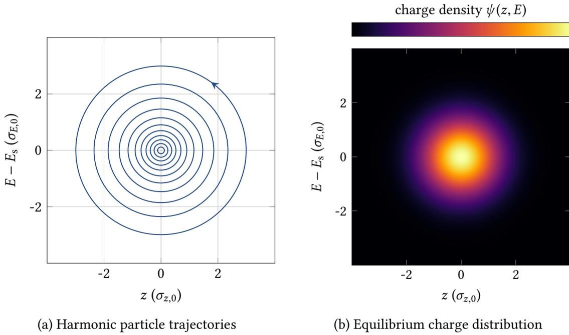
Figure 2.4.: (a) Driven by the restoring force of the RF system, off-momentum particles perform oscillations around the position and energy of the synchronous particle. (b) Radiation damping and quantum excitation lead to a Gaussian equilibrium distribution of particles in the longitudinal phase space.
