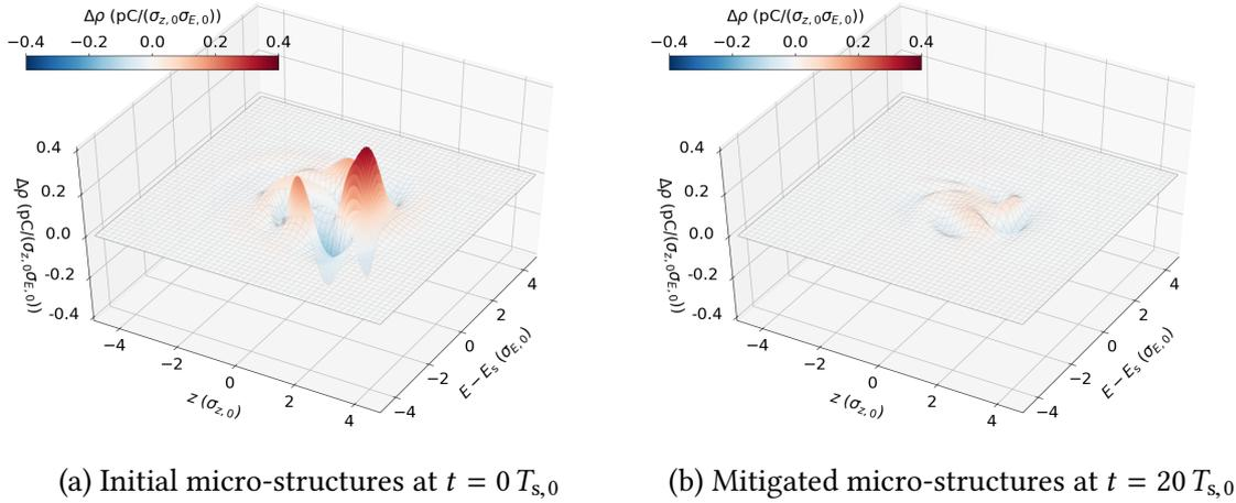
Figure 7.26.: (a) The natural micro-structures occurring at the beginning of the sequence displayed in Fig. 7.25 are quickly damped by the RL agent. (b) After 20 synchrotron periods, the micro-structures are significantly reduced in amplitude.
