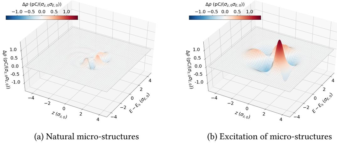
Figure 7.6.: (a) The naturally occurring set of micro-structures consists of about five structures with relatively small amplitudes. (b) An RF amplitude modulation at the third harmonic of the nominal synchrotron frequency,  $f_{\text{mod}} = 3.06 f_{s,0}$ , and with  $V_{\text{mod}} = 0.05 V_0$ , leads to a new set micro-structures in the longitudinal phase space, which consists of only three structures, but of much larger amplitude.
