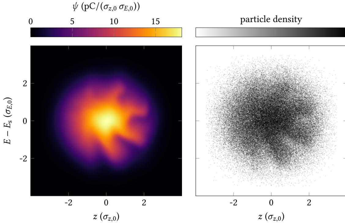
Figure 5.4.: In order to examine single particle trajectories, the initial charge distribution  $\psi(q, p, t_0)$  (left) is modeled by a distribution of one hundred thousand particles (right). The single particle motion is then simulated using the passive particle tracking implemented in Inovesa.
