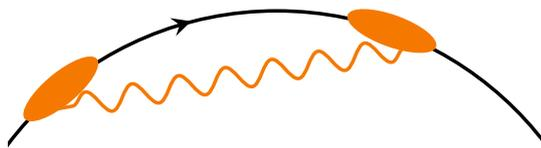
Figure 3.2.: The curved trajectory of an electron bunch in a bending magnet enables the self-interaction of the bunch with its own emitted CSR. By traveling on a straight line, the emitted photons can catch up with the electrons at the head of the bunch.
