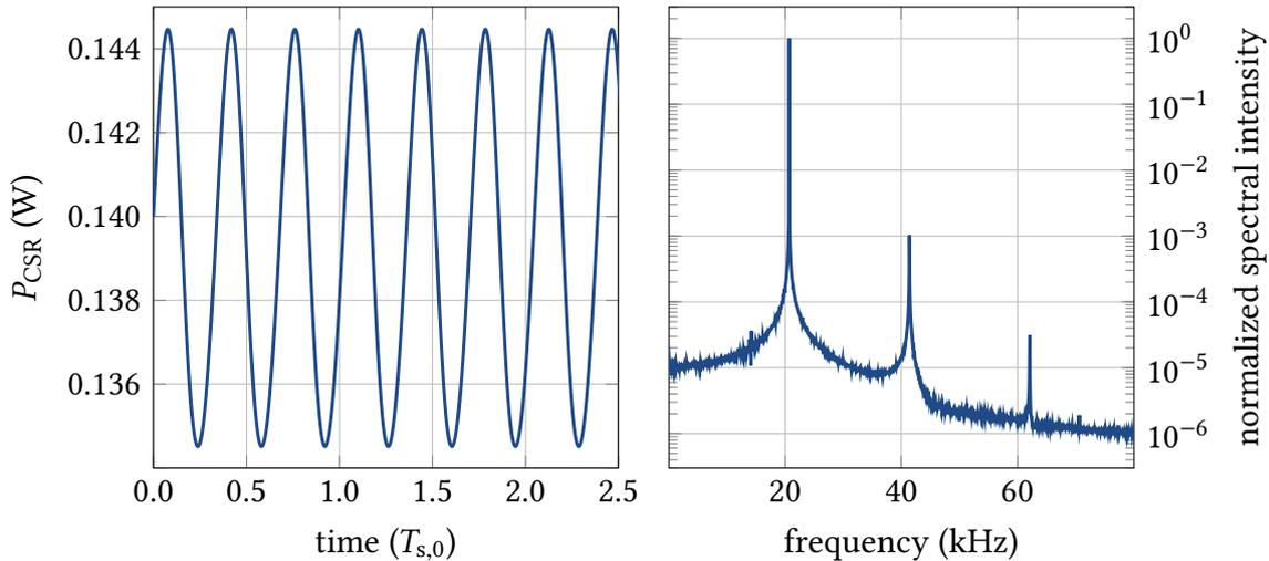
Figure 3.5.: CSR power time signal  $P_{\text{CSR}}(t)$  for the exemplary bunch current  $I = 115 \mu\text{A}$  (left) and the magnitude of its Fourier transform  $|\tilde{P}_{\text{CSR}}|$  (right).
