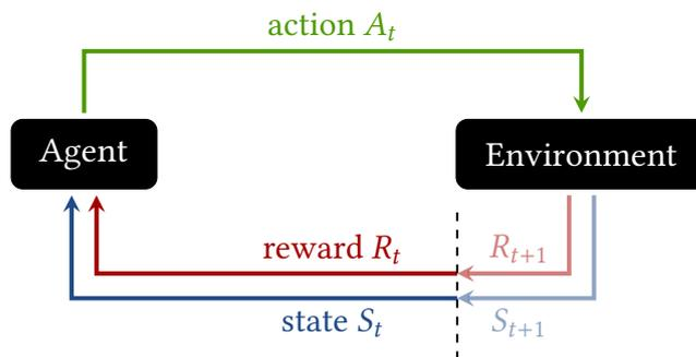
Figure 4.1.: Reinforcement learning is based entirely on the interaction between an agent and an environment. At each iteration, the agent receives a state  $S_t$  and reward  $R_t$  and executes an action  $A_t$ . Figure adapted from [48].
