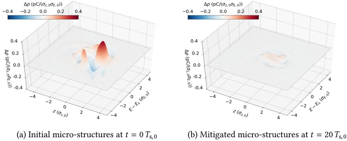
Figure 7.15.: (a) The initial micro-structures for the sequence displayed in Fig. 7.14 are quickly damped by the PPO agent. (b) Similarly to Fig. 7.9b, after 20 synchrotron periods, the micro-structures are clearly reduced in amplitude.
