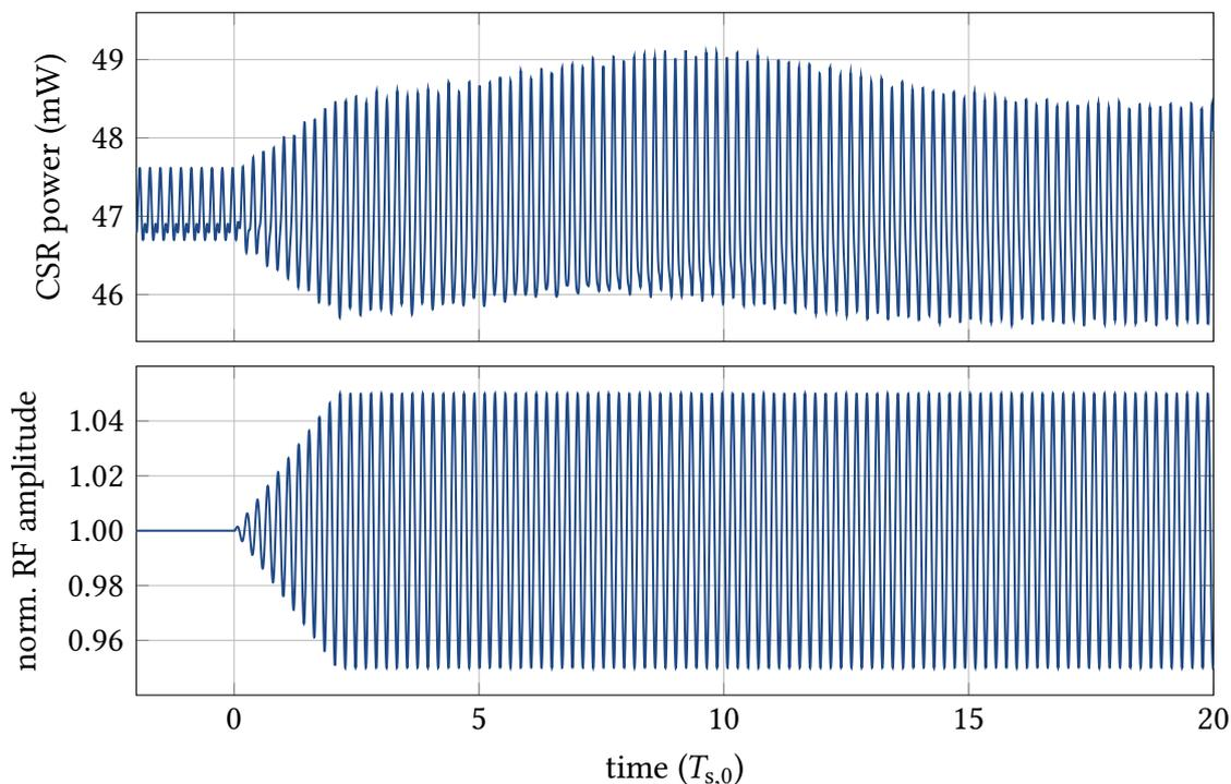
Figure 7.2.: The natural micro-bunching dynamics can be amplified with an RF amplitude modulation at the micro-structure frequency  $f_{\text{mod}} = f_{\text{ms}}$ . The oscillation of the CSR power signal (top) is immediately amplified by the RF modulation applied after  $t = 0 T_{s,0}$  (bottom). After an initial transition phase, roughly from  $t = 0 T_{s,0}$  to  $t = 15 T_{s,0}$ , the micro-bunching dynamics settle for a new quasi-equilibrium with higher oscillation amplitude.
