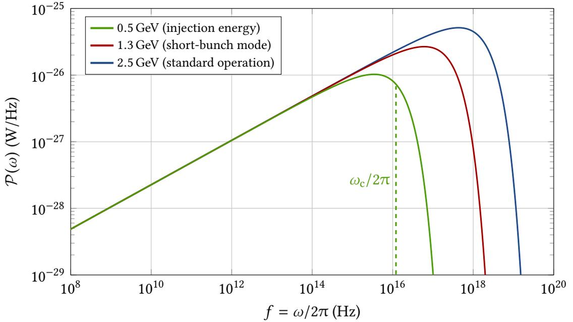
Figure 2.2.: Radiated power spectrum  $\mathcal{P}(\omega)$  of a single electron passing through a bending magnet ( $R = 5.559$  m) for the typical beam energies at KARA. The green dashed line marks the critical frequency  $\omega_c$  at injection energy, it divides the power spectrum into two sections of equal integrated radiation power.
