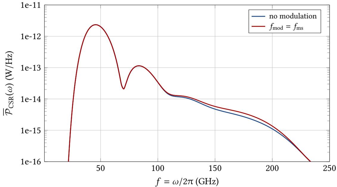
Figure 7.4.: The applied RF amplitude modulation amplifies the average CSR power spectrum in the frequency range corresponding to the spatial extent of the occurring micro-structures. Here, the emitted power is increased by up to 30 percent in the frequency range around 150 GHz.
