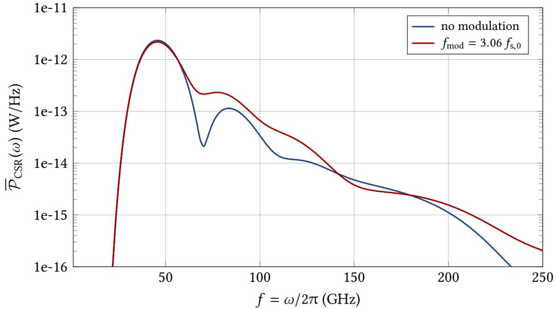
Figure 7.7.: The altered micro-bunching dynamics due to the applied RF amplitude modulation at  $f_{\text{mod}} = 3.06 f_{s,0}$  lead to substantial changes in the radiated CSR power spectrum. While the intensity is decreased in the frequency range corresponding to the spatial extent of the original micro-structure, the new set of large micro-structures shown in Fig. 7.6 increases the emission between 60 GHz and 140 GHz by a large margin.
