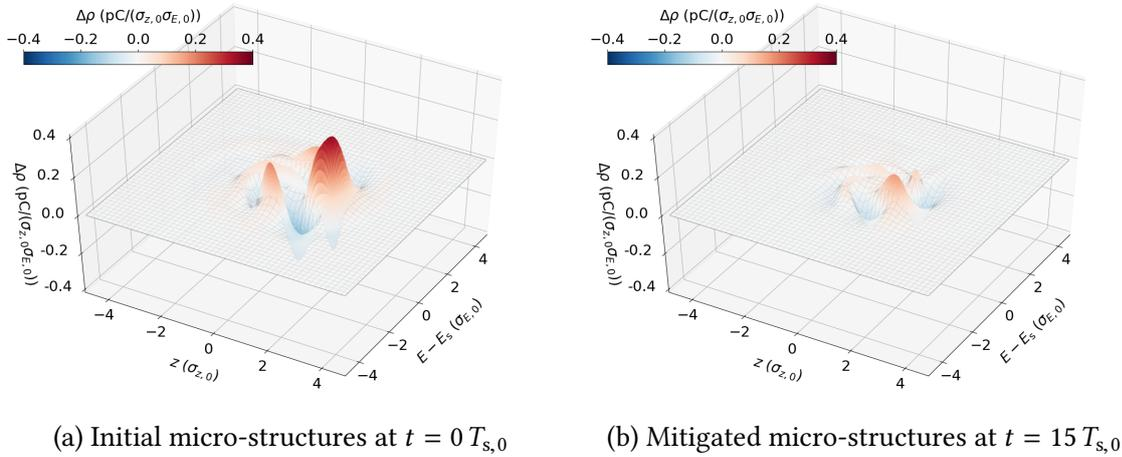
Figure 7.21.: (a) The initial micro-structures are damped by the DDPD agent during the sequence displayed in Fig. 7.20. (b) Shortly before the episode is terminated due to insufficient performance by the agent, the micro-structures are visibly reduced in amplitude.
