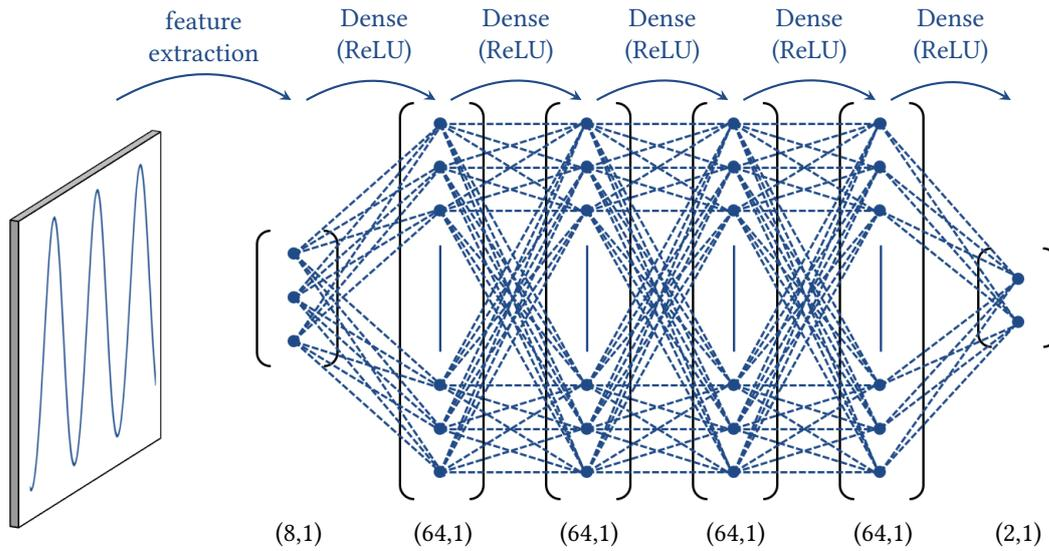
Figure 7.19.: Layout of the actor network used to process the observations defined by the eight-dimensional feature vector derived from the CSR power signal.
