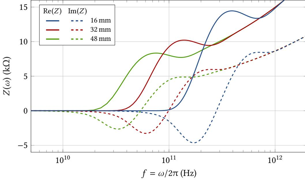
Figure 3.3.: CSR parallel plates impedance for different vacuum gaps. It describes the self-interaction of an electron bunch with its own emitted CSR under the shielding effect of the surrounding vacuum chamber walls. A reduced vacuum gap leads to a stronger shielding, which shifts the cut-off frequency due to the beam pipe to higher frequencies. The beam pipe installed at KARA has a total height of  $g = 32$  mm (red curves).
