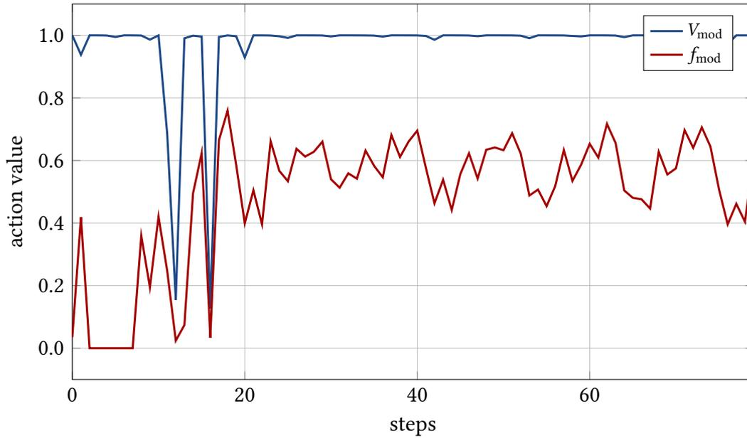
Figure 7.27.: Actions chosen by the PPO agent for the sequence displayed in Fig. 7.25. While the modulation frequency is dynamically adjusted according to the changing micro-bunching dynamics, the modulation amplitude is set close to the maximum value throughout the episode.
