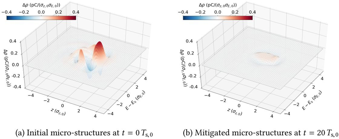
Figure 7.9.: (a) The initial micro-structures for the sequence displayed in Fig. 7.8 are quickly damped by the applied modulation of the RF amplitude. (b) After 20 synchrotron periods, the micro-structures are mitigated significantly, which yields a smooth charge distribution in the longitudinal phase space.
