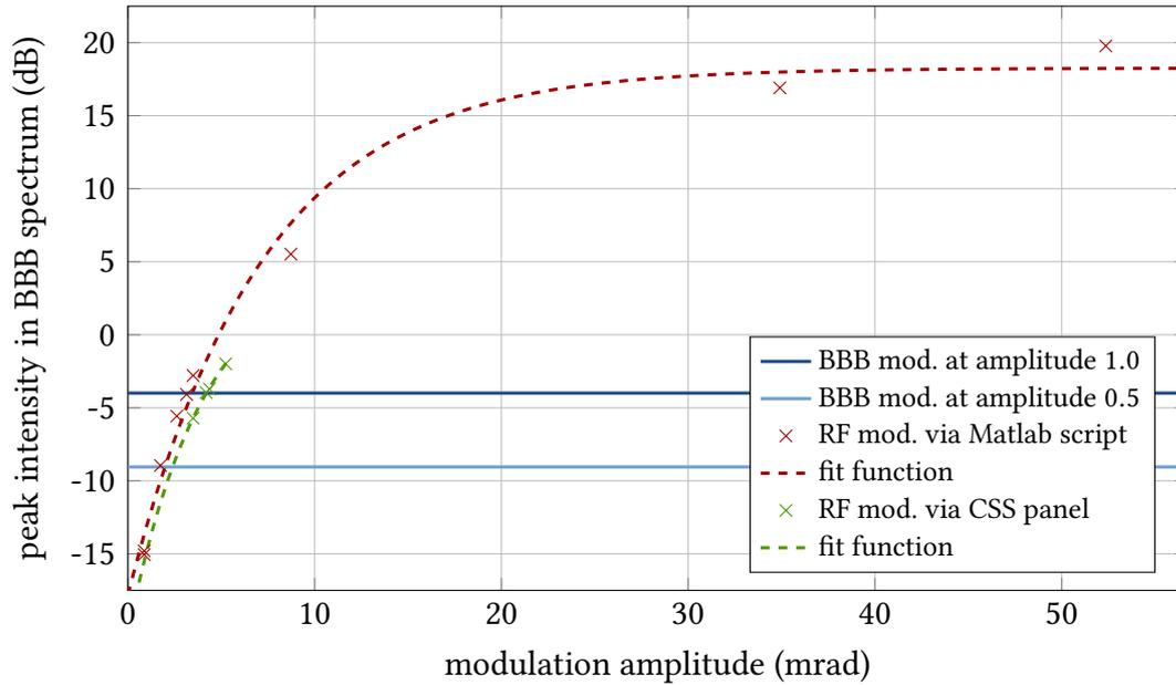
Figure 8.2.: Estimate of the BBB cavity voltage. By comparing the effect of RF phase modulations via the main RF system and the BBB system, the maximum BBB cavity voltage can roughly be estimated using Eq. (8.2). The measurements are interpolated by fitting a limited growth function,  $f(x) \doteq a - (a - b)e^{-cx}$ . Data: Courtesy of Edmund Blomley.
