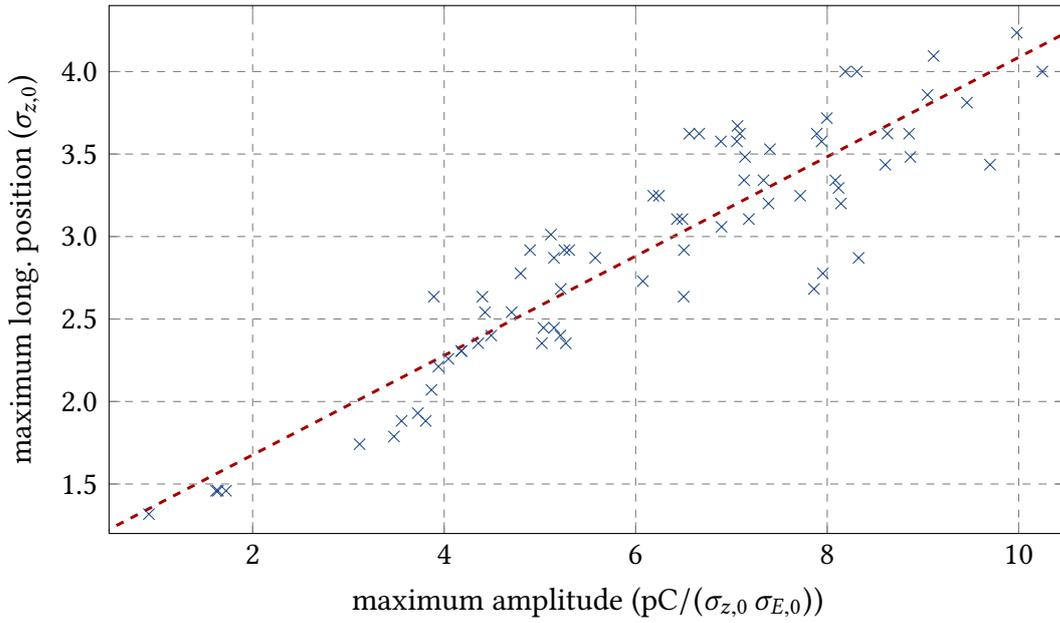
Figure 5.12.: Correlation between the maximum amplitude and maximum longitudinal position of the occurring micro-structures. Shown is simulation data for bunch currents between 260  $\mu\text{A}$  and 1000  $\mu\text{A}$ . The dashed red line illustrates the clear linear correlation with a correlation coefficient of 0.91.
