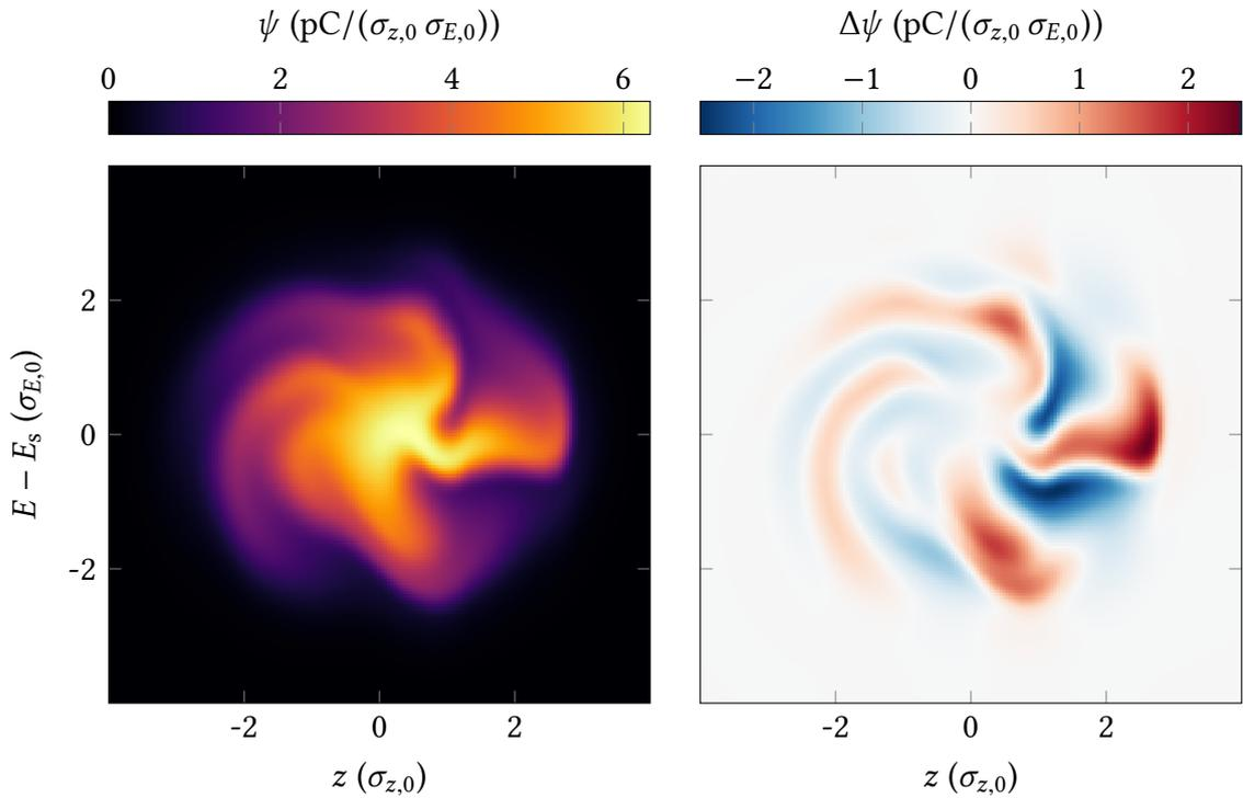
Figure 3.10.: Snapshot of the charge distribution in phase space in the sawtooth bursting regime (left). The subtraction of the temporal average reveals very similar micro-structures compared to Fig. 3.8, though with a significantly larger amplitude (right).
