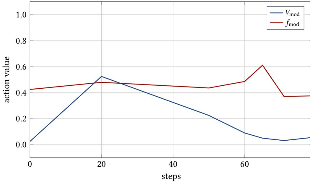
Figure 7.10.: Action values chosen during the sequence displayed in Fig. 7.8. The modulation amplitude  $V_{\text{mod}}$  is initially increased until the actions show the desired effect and the perturbation by the CSR wake potential is reduced. After the first 20 steps, it can therefore be lowered again. The modulation frequency is kept close to the natural micro-structure frequency at  $f_{\text{ms}} = 2.99 f_{s,0}$ .
