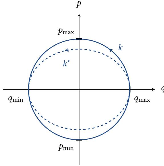
Figure 5.1.: A small perturbation of the strength of the restoring force  $k$  leads to an elliptical particle trajectory in the phase space spanned by the generalized coordinates  $q$  and  $p$ .
