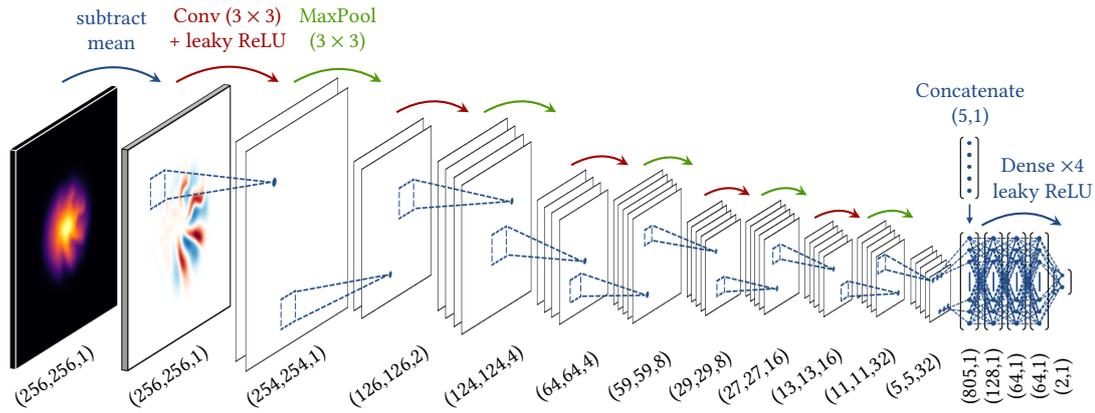
Figure 7.13.: Layout of the actor network used to process the states defined by Eq. (6.27). The charge density matrix is processed by alternating convolution and max pooling layers and subsequently concatenated with the additional feature vector, which serves as the input for the final fully connected layers.
