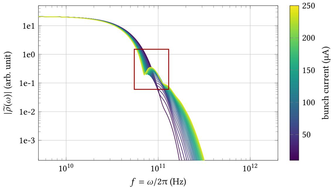
Figure 5.7.: Magnitude of the Fourier transformed bunch profile  $|\tilde{\rho}(\omega)|$  for a range of bunch currents below the instability threshold of  $I_{\text{th}} = 260 \mu\text{A}$ . The red rectangle marks the additional frequency component (at roughly 85 GHz) that is excited due to the perturbation by the CSR wake potential.
