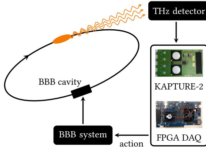
Figure 8.1.: Planned hardware implementation of the proposed RL feedback scheme. The CSR power signal is measured by a THz detector, sampled by the KAPTURE-2 board and read out by the FPGA DAQ board, on which the RL algorithm is implemented. The chosen action is passed to the BBB control system, which generates the corresponding modulation of the RF amplitude. Images: Courtesy of Weijia Wang.
