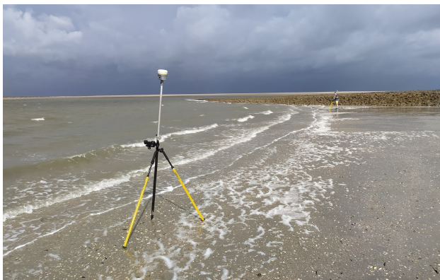
Figure 3. GNSS survey during the F-SAR flight mission. Direction of view towards north. Note the (in this case already scattered) sea foam as indicator for the WLB.
