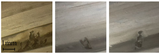
Fig. 1 Examples of pittings on the spindle. All images have the same original size and ration hence the scale bar and the ratios are easily transferable to all other images
