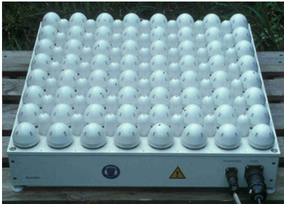
Fig. 23.4 Phased-array sodar with 64 sound transducers and no enclosure (photo © Helmut Mayer)
