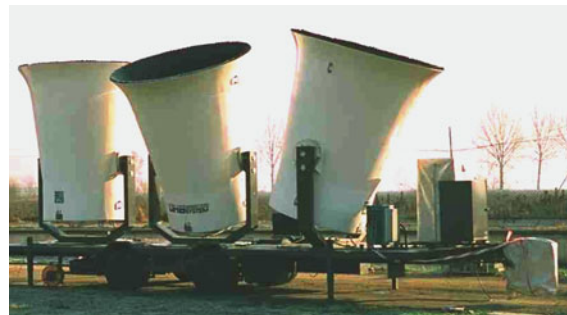
Fig. 23.3 Sodar with three antennas (horns) (photo © Stefan Emeis)
