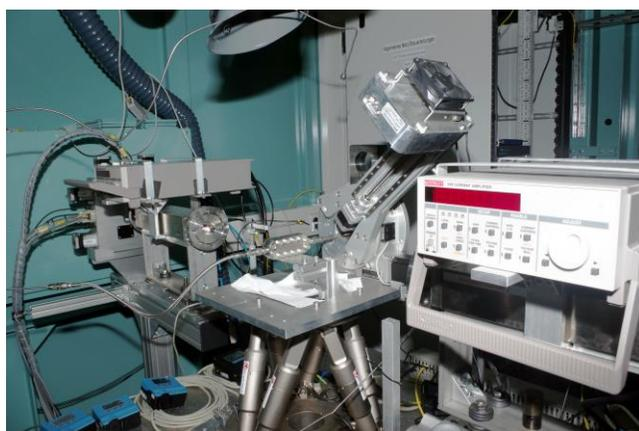
**Figure 8:** Side view of the X-ray transmission experiment with the flow cell attached to the hexapod for positioning and steel-jacketed tubing for connection to the reaction equipment.
