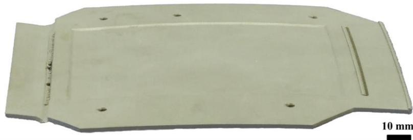
Figure 4.11. Additively manufactured 2 mm thick PMS plate created with the same laser parameters and scan strategy like the test specimen in figure 4.2.
