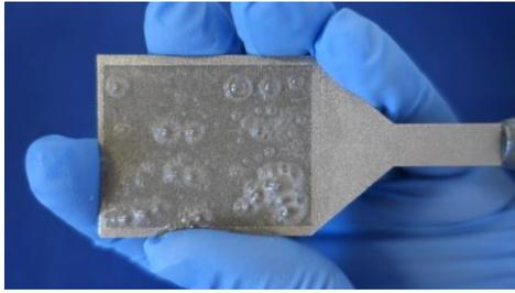
Figure A. 4. Samples with internal channels printed by porous-dense composite.
