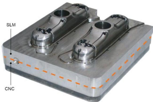
Figure 1.8. Die-casting dies with conformal cooling channels manufactured by a LB-PBF printer and a CNC machine [94].
