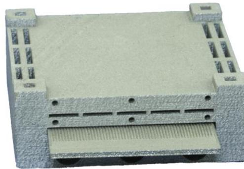
Figure 4.31. Additively manufactured temperature barrier test reactor with microchannel plate.
