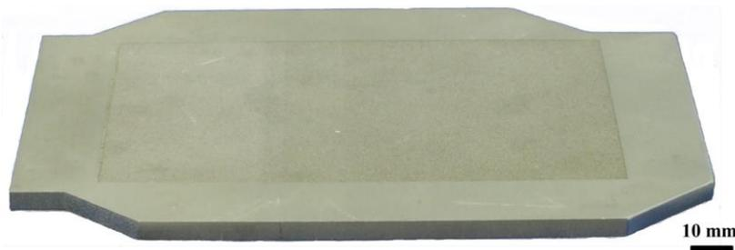
Figure 4.12. Additively manufactured 5 mm thick PMS plate.
