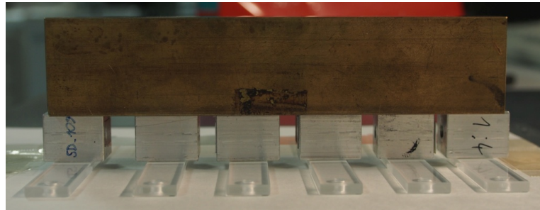
Figure 4.21: Sample preparation for underfill radiation hardness tests.
