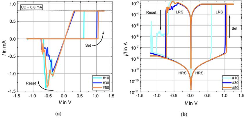
**Figure 4.5:**  $I - V$  curves of the inkjet-printed memristor, which shows a bipolar-switching behavior. For the set process, a compliance current of 0.8 mA is used. Furthermore, ECM-cell type switching behavior is observable. **(a)**  $I - V$  curves on a linear scale, showing cycle number ten, 30 and 50. **(b)**  $I - V$  curves on a semi-logarithmic scale, showing cycle number ten, 30 and 50. Adapted from [203], © 2021 AIP Publishing.
