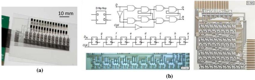
**Figure 2.4:** Advanced circuits based on printed TFTs. (a) Printed OTFT-based address decoder and ferroelectric memory on flexible substrate, connected with rigid printed circuit board (PCB) [88]. Reproduced under CC BY-NC-ND 3.0 license, <https://creativecommons.org/licenses/by-nc-nd/3.0/>. (b) Electrochemically-gated transistors deployed in addressing circuitry for an integrated electrochromic display [93]. Reproduced under CC BY 4.0 license, <https://creativecommons.org/licenses/by/4.0/>.
