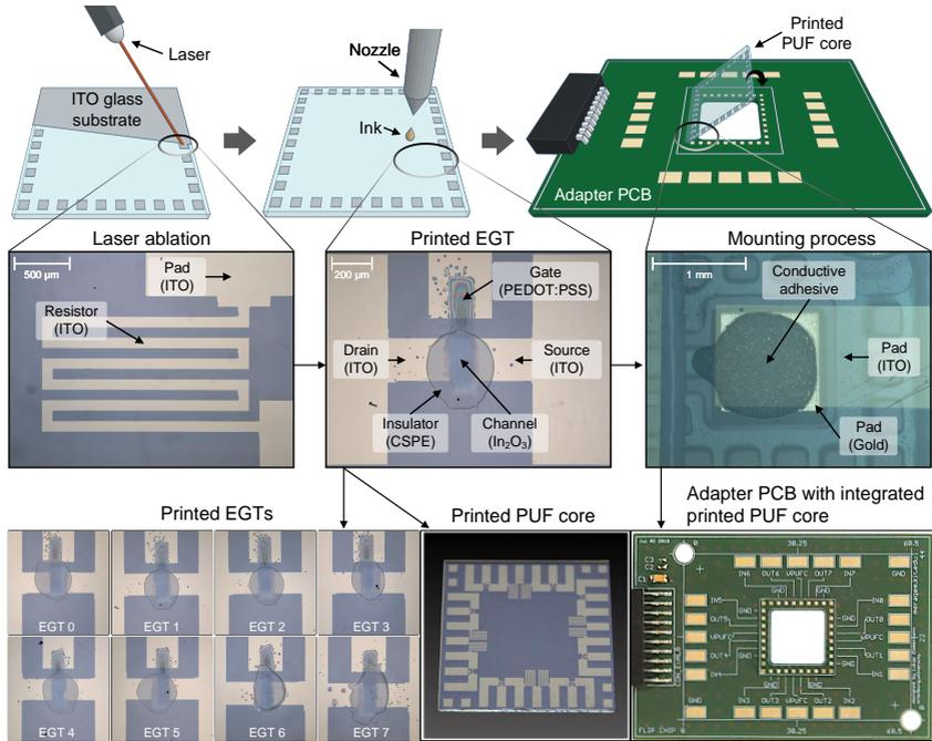
**Figure 6.8:** Fabrication and integration workflow of the PE-based DiffC-PUF core on the adapter PCB, from left to right. Furthermore, additional images are shown, such as microscopic images of eight EGTs on a printed PUF core, a standalone printed PUF core on glass substrate and the integrated PUF core on the adapter PCB. Adapted from [200] under CC BY 4.0 license, <https://creativecommons.org/licenses/by/4.0/>.
