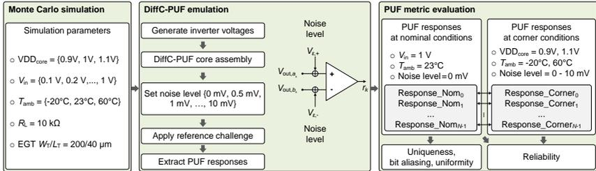
**Figure 5.15:** DiffC-PUF simulation methodology including noise level allocation and simulation parameter. Adapted from [129], ©2019 IEEE.
