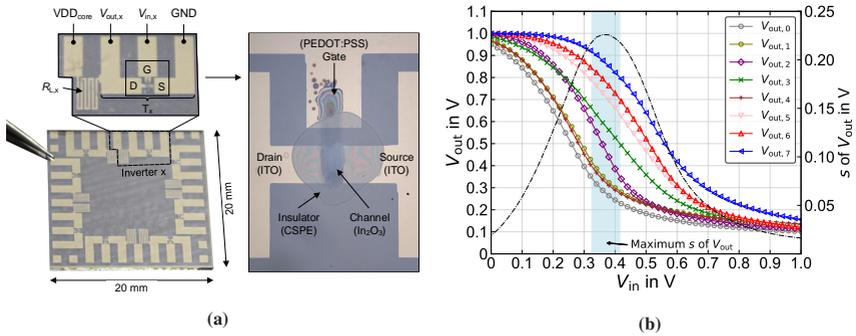
**Figure 5.22:** PE-based DiffC-PUF core on glass substrate. **(a)** Photograph of the fabricated DiffC-PUF core. **(b)** Measured inverter transfer curves, including the standard deviation of the incorporated inverters  $V_{out}$ . Adapted from [129], © 2019 IEEE.
