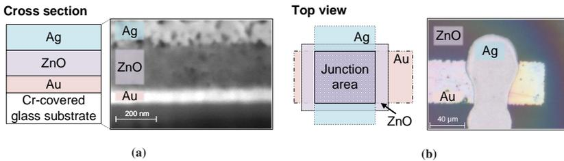
**Figure 4.3:** Schematic and optical images of the inkjet-printed memristor stack. **(a)** Cross section of the memristor material stack. The optical image was obtained via FIB-SEM. **(b)** Top view of the device, visualizing the crossing junction. The optical image clearly shows the different material layers from a top view. The ZnO is covering an extended surface area. Adapted from [203], © 2021 AIP Publishing.
