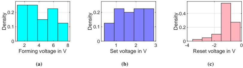
**Figure 4.7:** Device-to-device variability for the forming, set and reset voltages, plotted as histogram over 40 devices. (a) Forming voltage. (b) Set voltage. (c) Reset voltage. Adapted from [203], © 2021 AIP Publishing.
