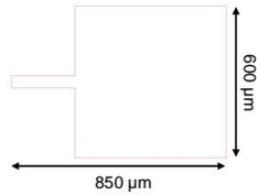
**Figure A.3:** Inkjet-printed memristor bottom electrode layout.
