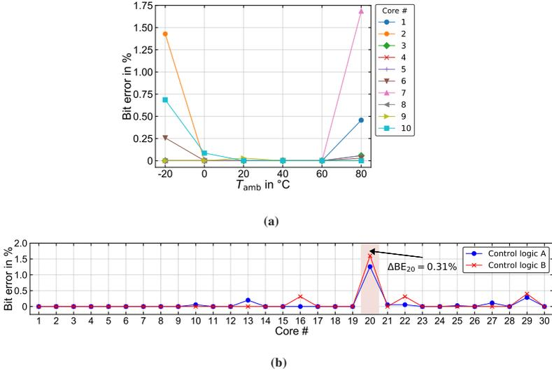
**Figure 6.7:** Measured Si-based DiffC-PUF bit errors. (a) BE of 10 DiffC-PUF cores, visualized over  $T_{amb}$ . (b) BE of 30 DiffC-PUF cores over two deployed control logic boards (A and B). Adapted from [138] under CC BY 4.0 license, <https://creativecommons.org/licenses/by/4.0/>.
