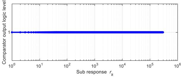
**Figure 6.3:** Comparator output, over the corresponding 298,200 sub-responses  $r_k$ , during the prolonged continuous cycling test.
