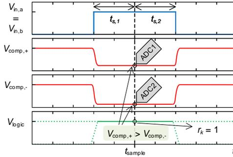
**Figure 6.2:** Schematic readout timing setup for the voltage levels and the corresponding output bit. Adapted from [138] under CC BY 4.0 license, <https://creativecommons.org/licenses/by/4.0/>.
