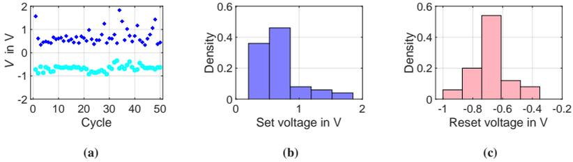
**Figure 4.6:** Cycle-to-cycle variability for a single device over 50 repetitions. The initial forming voltage was 5.17 V. (a) Set and reset voltage variation over 50 cycles. (b) Set voltage variation visualized as histogram. (c) Reset voltage visualized as histogram. Adapted from [203], © 2021 AIP Publishing.
