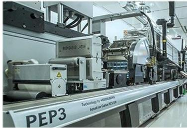
**Figure 2.1:** Pilot printing line "Gallus RCS 330", using conventional printing methods for PE. Source: Innovationlab GmbH.
