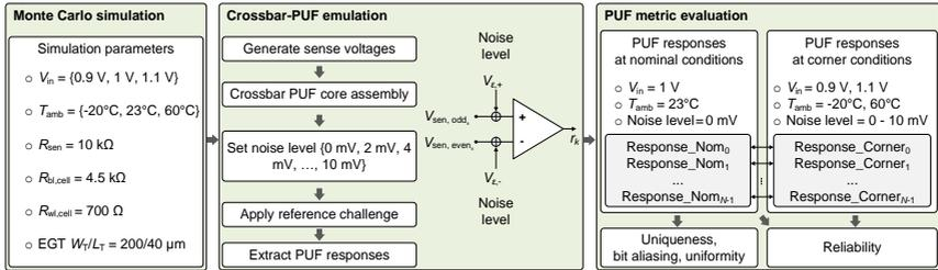
**Figure 5.8:** Printed crossbar PUF simulation methodology including noise level allocation and simulation parameter. Adapted from [129], ©2019 IEEE.
