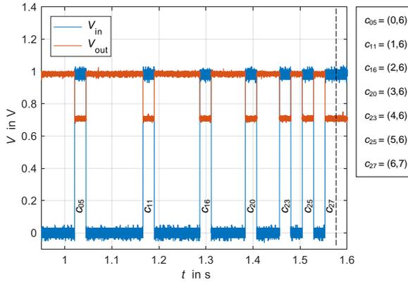
**Figure 6.4:** Exemplary input and output voltages of inverter number six of an arbitrary Si-based DiffC-PUF core. The corresponding sub-challenge  $c_k$ , which is used to address inverter number six is labeled. The end of the CRP cycle is marked with the vertical black dashed line.
