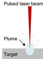
**Figure 2.3:** Conceptual, simplified schematic of a laser ablation process.
