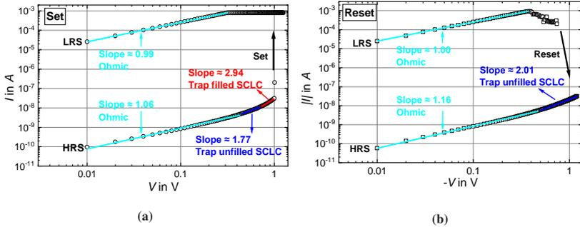
**Figure 4.9:** Double-logarithmic  $I - V$  plot for conduction mechanism investigation. (a) Set process investigation including the linear fitted curves and corresponding slopes over different voltage regions. (b) Reset process investigation, including the linear fitted curves and corresponding slopes, over different voltage regions. Adapted from [203], © 2021 AIP Publishing.
