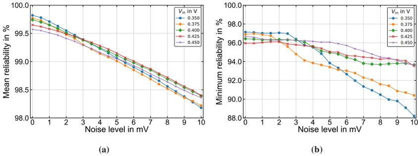
**Figure 5.21:** DiffC-PUF reliability over  $V_{in} = \{0.35 \text{ V}, 0.375 \text{ V}, \dots, 0.45 \text{ V}\}$  and NL. (a) Mean reliability. (b) Minimum reliability. Adapted from [129], © 2019 IEEE.
