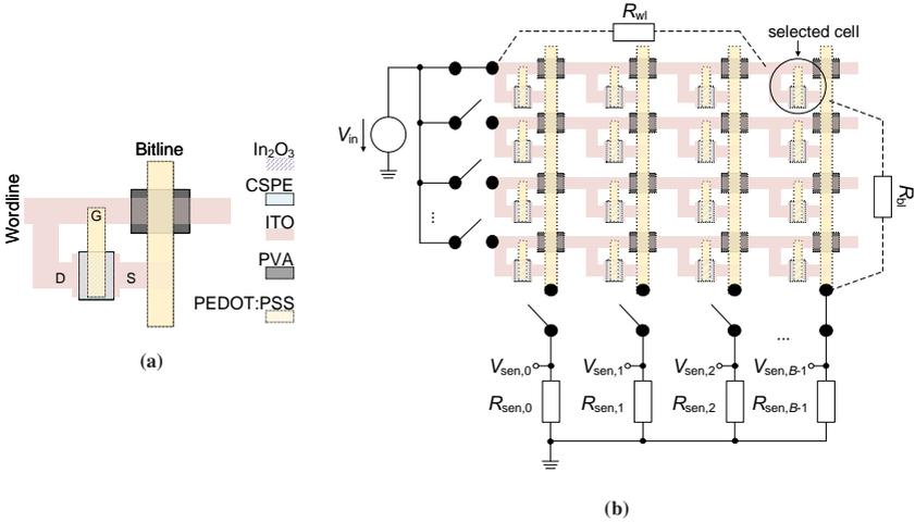
**Figure 5.6:** Printed crossbar layout. **(a)** Layout for crossbar integrated, diode-connected, EGT cell. The drain (D), gate (G) and source (S) terminals are labeled. **(b)** Diode-connected EGT crossbar single cell biasing scheme. Adapted from [219], © 2021 IEEE.
