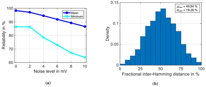
**Figure 5.10:** Printed crossbar PUF reliability and uniqueness evaluation. **(a)** Mean and minimum reliability including noise levels, ranging from 0 mV to 10 mV. **(b)** The printed crossbar PUF uniqueness is  $\mu_{\text{inter}} = 49.84\%$  with a standard deviation of  $\sigma_{\text{inter}} = 18.26\%$ . Adapted from [219], © 2021 IEEE
