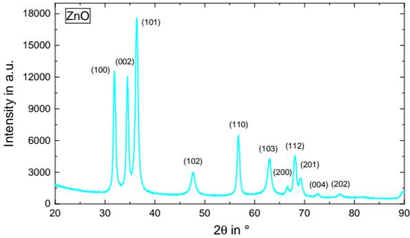
**Figure 4.4:** X-ray powder diffraction results of the poly-crystalline ZnO film, formed from the inkjet-printed zinc-nitrate precursor salt. Adapted from [203], © 2021 AIP Publishing.
