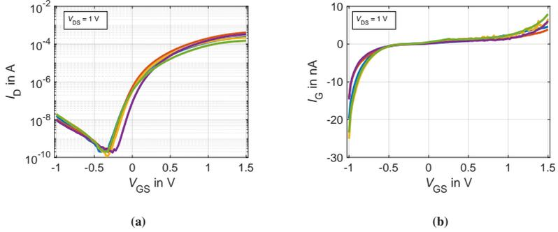
**Figure 4.2:** Measured transfer curves and corresponding gate leakage of five EGTS with a channel width  $W_T = 200 \mu\text{m}$  and length  $L_T = 60 \mu\text{m}$  at  $V_{DS} = 1$  V and RH = 50 %. (a) Transfer curves of the measured EGTS, with  $I_D$  plotted in logarithmic scale. (b) The corresponding gate leakage currents.
