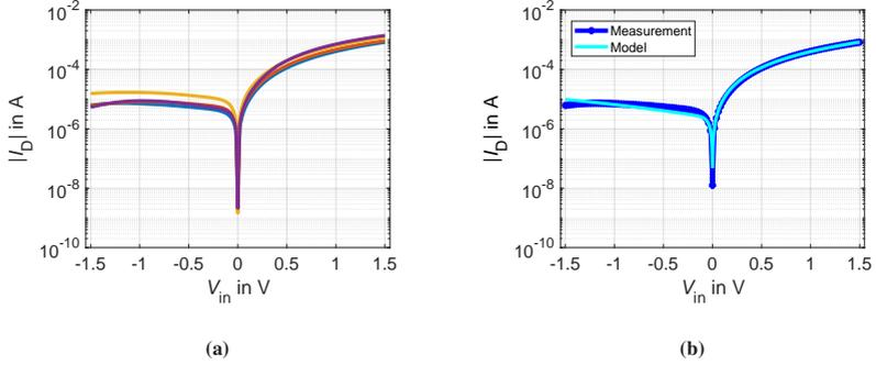
**Figure 5.2:** Near-zero threshold voltage, diode-connected EGT  $I - V$  curves plotted on semi-logarithmic scale over the absolute drain current and EKV model fit. **(a)** Four measured diode-connected near-zero  $V_{th}$  EGT  $I - V$  curves with a channel width  $W_T = 200 \mu\text{m}$  and length  $L_T = 90 \mu\text{m}$  at  $\text{RH} = 60\%$ . **(b)** Fitted EKV model curve over one of the measured diode-connected EGT. Adapted from [80], © 2020 IEEE.
