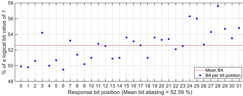
**Figure 5.11:** Printed crossbar PUF bit aliasing plotted over each response bit position, including the mean bit aliasing.
