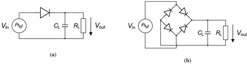
**Figure 3.1:** Basic passive rectifier circuit schematics, including a capacitor for rectified voltage smoothing and a resistive load. **(a)** Schematic for a half-wave rectifier, incorporating a single diode. **(b)** Schematic for a full-wave rectifier, incorporating four diodes.
