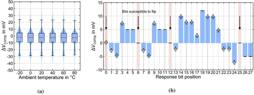
**Figure 6.5:** Si-based DiffC-PUF comparator input voltage differences  $\Delta V_{\text{comp}}$ . **(a)**  $\Delta V_{\text{comp}}$  of ten PUF cores over temperature. **(b)**  $\Delta V_{\text{comp}}$  per response bit of one selected PUF core (no. 20). Adapted from [138] under CC BY 4.0 license, <https://creativecommons.org/licenses/by/4.0/>.
