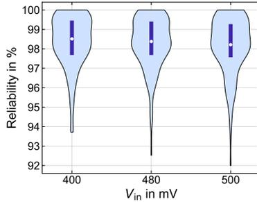
**Figure 5.20:** DiffC-PUF reliability distribution over  $V_{in} = \{0.4 \text{ V}, 0.48 \text{ V}, 0.5 \text{ V}\}$ , visualized as violin plot. Adapted from [129], © 2019 IEEE.
