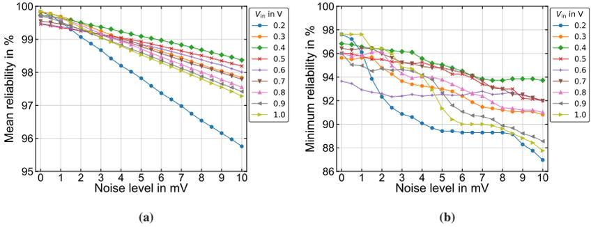
**Figure 5.18:** DiffC-PUF reliability over  $V_{in}$  and NL. (a) Mean reliability. (b) Minimum reliability. Adapted from [129], © 2019 IEEE.
