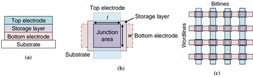
**Figure 3.2:** Conceptual memristor schematics. (a) Cross section of a memristor material stack. (b) Top-view of a basic resistive switching device stack including the junction area in which resistive switching occurs, based on the overlap in bottom electrode ( $w$ ) and top electrode ( $l$ ). (c) Memristors arranged in a crossbar architecture.
