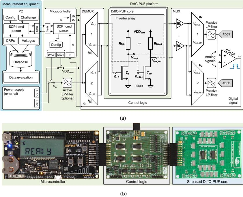
**Figure 6.1:** DiffC-PUF as a holistic embedded platform in a schematic view and as photograph. (a) Schematic for the DiffC-PUF, including the required peripherals for CRP generation. (b) Photograph of the DiffC-PUF as platform incorporating the EFM32LG-STK3600 development board, the control logic and Si-based PUF core. Adapted from [138] under CC BY 4.0 license, <https://creativecommons.org/licenses/by/4.0/>.
