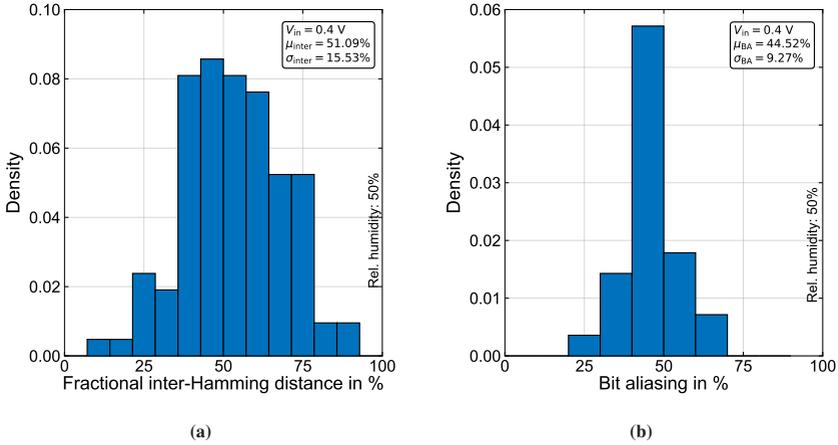
**Figure 6.11:** PE-based DiffC-PUF uniqueness and bit aliasing. (a) PE-based DiffC-PUF uniqueness. (b) PE-based DiffC-PUF bit aliasing. Adapted from [200] under CC BY 4.0 license. <https://creativecommons.org/licenses/by/4.0/>.
