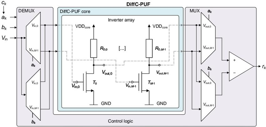
**Figure 5.14:** System architecture of the DiffC-PUF, including the inverter-based PUF core and the Si-based control logic. Adapted from [138] under CC BY 4.0 license, <https://creativecommons.org/licenses/by/4.0/>.
