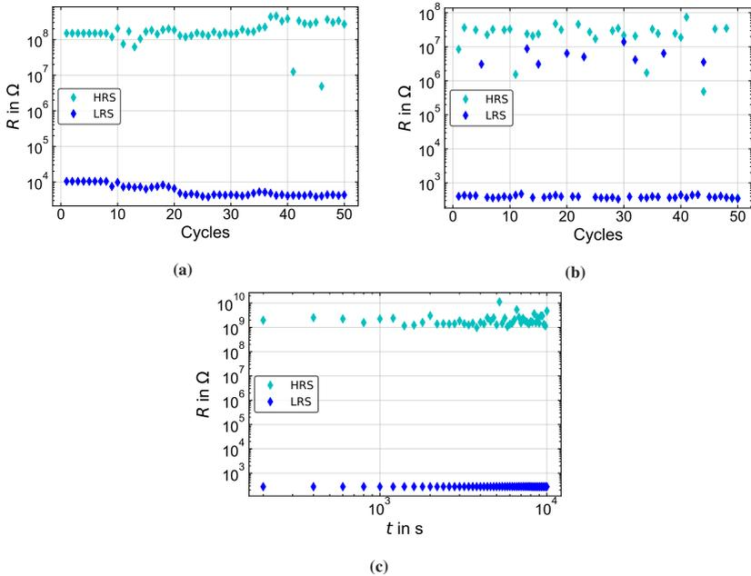
**Figure 4.8:** Endurance and retention test results of the printed device. (a) Endurance test using DC sweep cycling over 50 cycles. (b) Endurance test using pulse voltage cycling over 50 cycles. (c) Retention test over  $10^4$  s time period over the HRS and LRS, respectively. Adapted from [203], © 2021 AIP Publishing.
