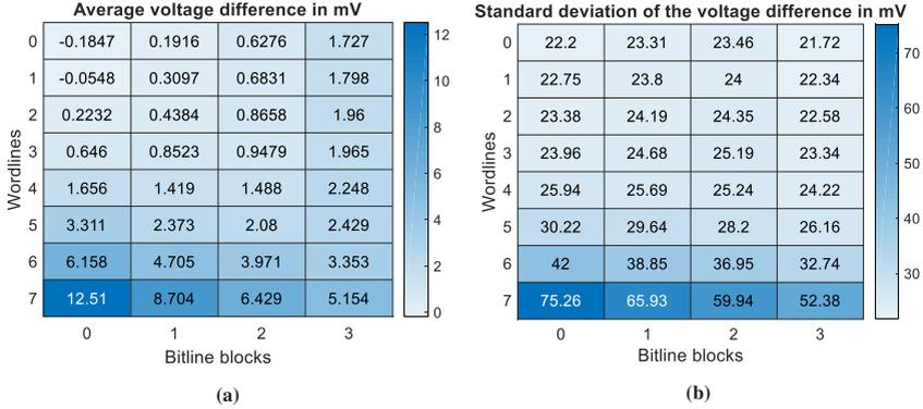
**Figure 5.9:** Voltage difference ( $\Delta V_{\text{sen}}$ ) investigations. **(a)** Average voltage difference of each bitline block. **(b)** Standard deviation of the voltage difference.
