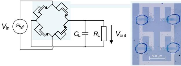
**Figure 5.3:** Schematic for the diode-connected EGT full-wave rectifier, including the externally connected capacitor and resistive load. The light blue shaded area marks the inkjet-printed part. A microscopic image of the inkjet-printed full-wave rectifier is shown. Adapted from [80], © 2020 IEEE.
