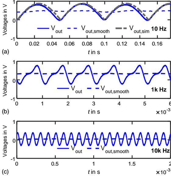
**Figure 5.4:** Frequency dependency of the full-wave rectifier. (a) Rectifier output voltages  $V_{out}$ ,  $V_{out,smooth}$  and  $V_{out,sim}$ . (b) Rectifier output voltage at 1 kHz. (c) Rectifier output voltage at 10 kHz. Adapted from [80], © 2020 IEEE.
