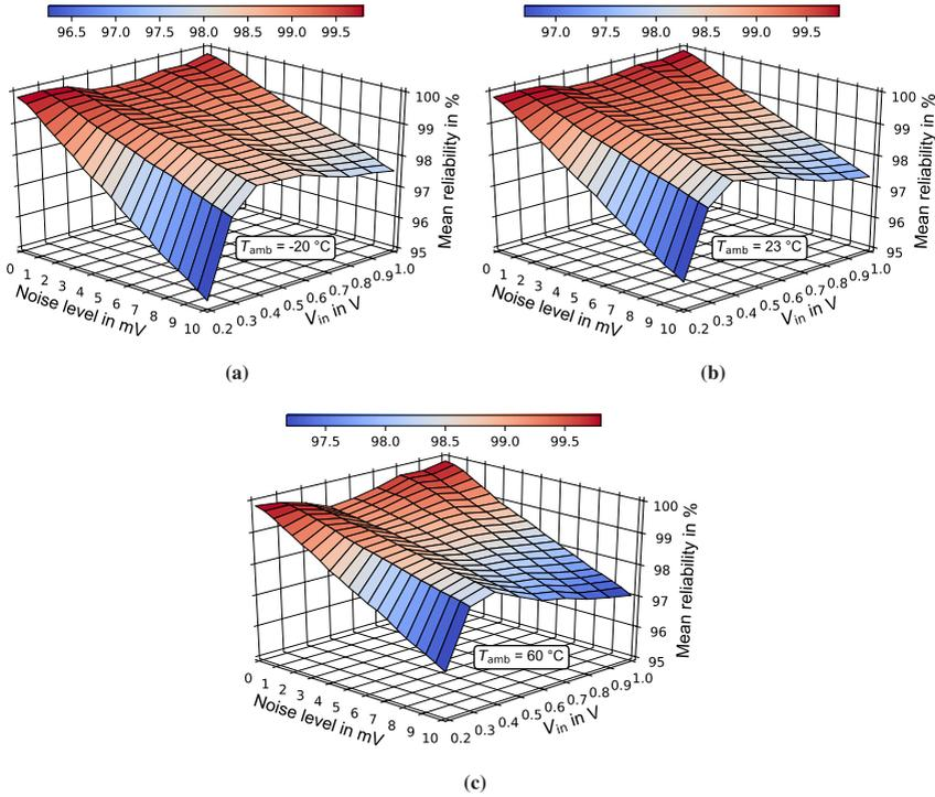
**Figure 5.17:** DiffC-PUF reliability over noise levels and temperature, visualized as surface plot. (a) Reliability surface plot at  $-20^\circ\text{C}$ . (b) Reliability surface plot at  $23^\circ\text{C}$ . (c) Reliability surface plot at  $60^\circ\text{C}$ . Adapted from [129], © 2019 IEEE.
