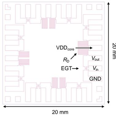
**Figure A.1:** PE-based DiffC-PUF core signal routing layer layout.
