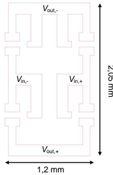
**Figure A.2:** Full-wave rectifier signal routing layer layout.
