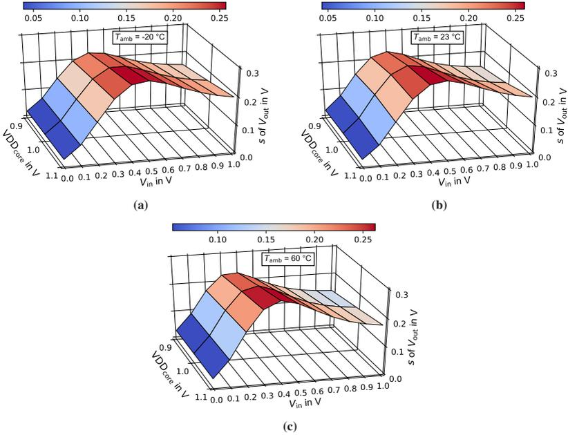
**Figure 5.16:** Standard deviation  $s$  of  $V_{out}$  over  $T_{amb} = \{-20^\circ\text{C}, 23^\circ\text{C}, 60^\circ\text{C}\}$ ,  $V_{in}$  and  $VDD_{core}$ , visualized as surface plot. (a) Surface plot at  $-20^\circ\text{C}$ . (b) Surface plot at  $23^\circ\text{C}$ . (c) Surface plot at  $60^\circ\text{C}$ . Adapted from [129], © 2019 IEEE.
