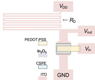
**Figure 5.13:** Inverter incorporating resistive ITO strip and EGT, including probing pad labels.
