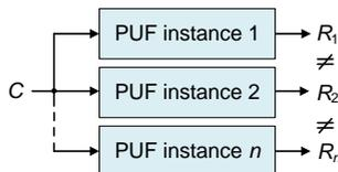
**Figure 3.4:** Schematic for response  $R$  generation over different PUF instances of the same type, stimulated with an identical challenge  $C$ . Due to intrinsic, unpredictable PUF instance behavior, the output response differs for each PUF instance.
