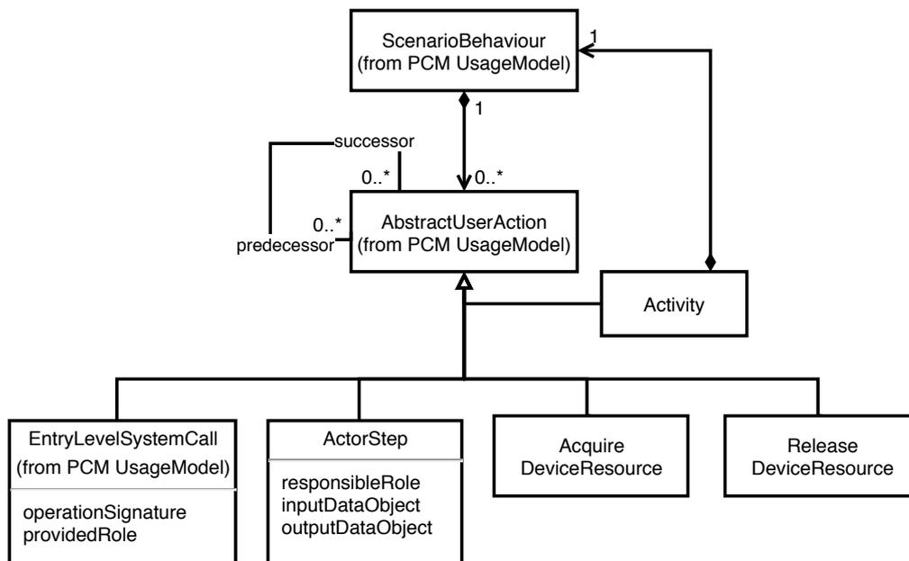
**Figure 2.16:** Shows an excerpt of the metamodel of IntBIIS regarding the integration of business processes into PCM [105].
