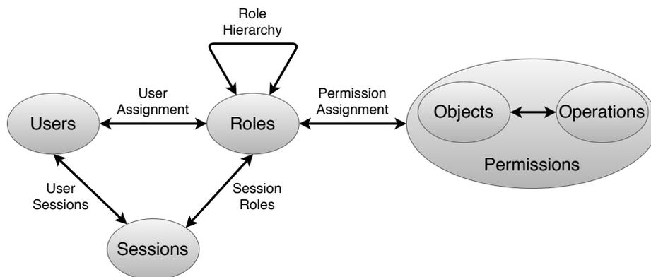
**Figure 2.7:** The reference model of the hierarchical RBAC [2].
