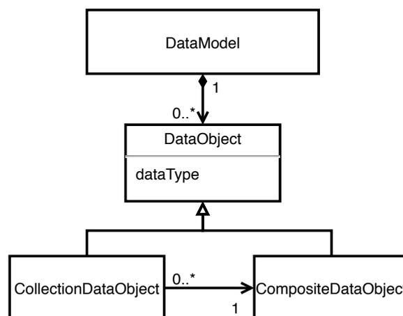
**Figure 2.18:** Shows the metamodel of IntBIIS regarding the integration of data objects into PCM [105].
