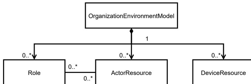
**Figure 2.17:** Shows the metamodel of IntBIIS regarding the integration of actor resources into PCM [105].
