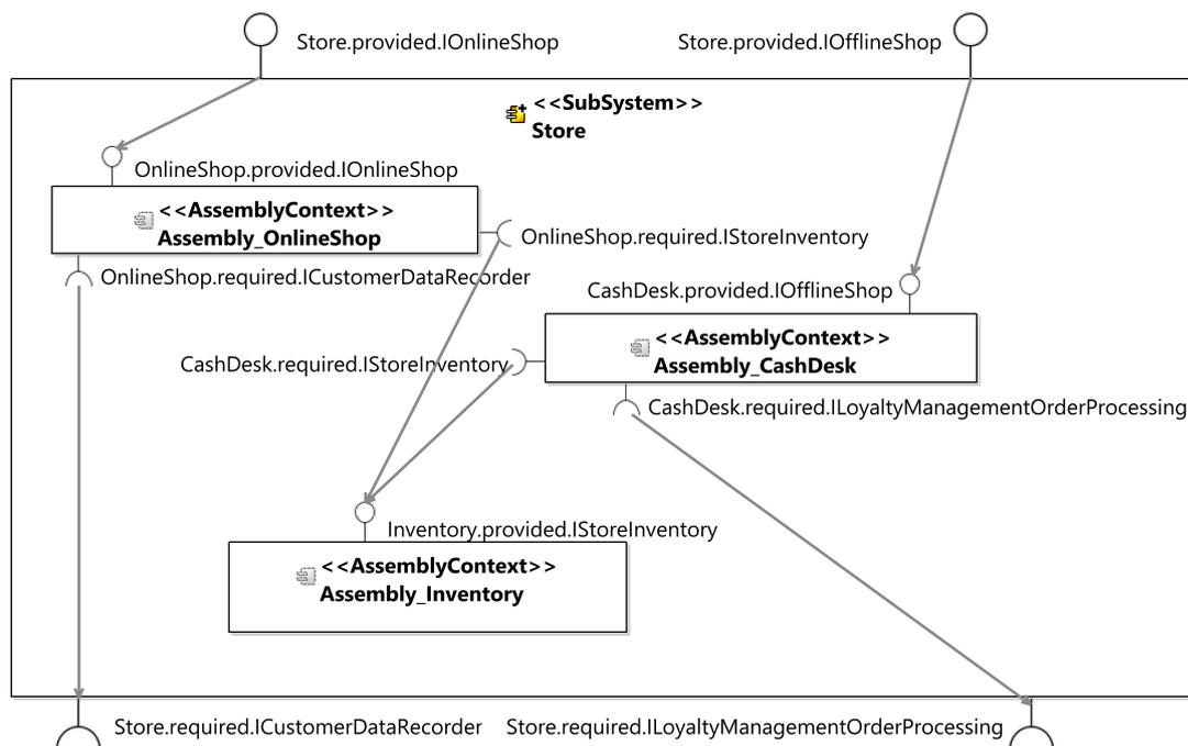
**Figure 3.38:** Shows the components of the system *Store*.
