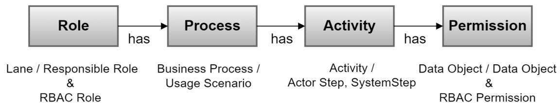
**Figure 3.9:** Shows the ACR mapping model filled by BAcsTract and PAcsTract during the extraction of ACRs from business processes.
