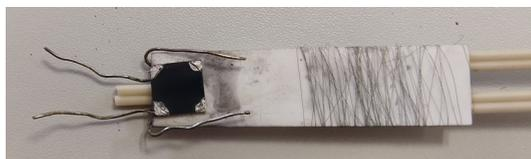
**Figure 5.** Conductance measurement system with a REBCO sample mounted and contacted.
