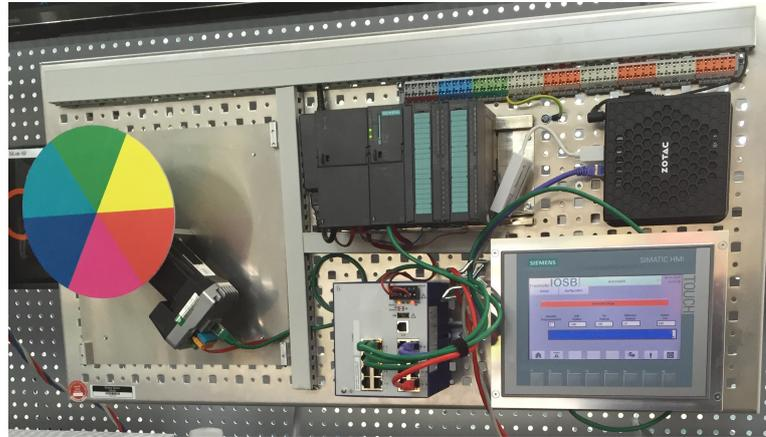
**Figure 11.4:** Hardware components of the system to be verified. Image provided by Fraunhofer IOSB
