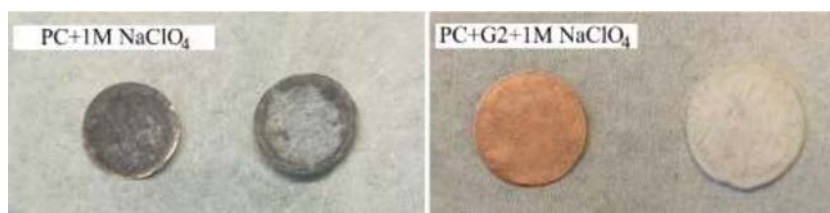
Fig. 13. Images of Cu electrode and separators after disassembling the Cu/Na cells from plating-stripping experiments, exemplarily shown for “PC+1 M NaClO 4 ” and “PC+G2+1 M NaClO 4 ”.
