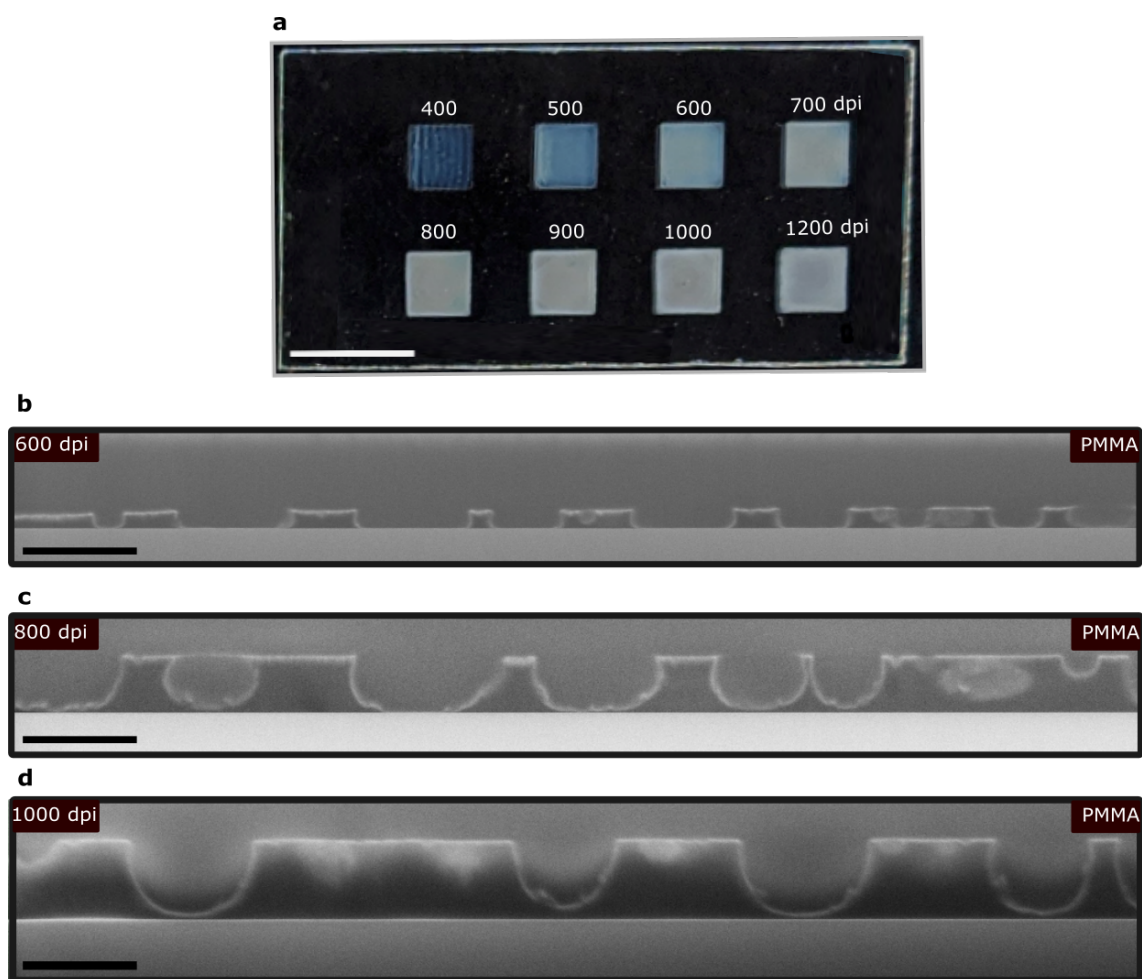
Figure 4.11. Influence of the printed pixel thickness on the nanoscale morphology of the phase-separated polymer films. a) Photograph of pixels printed at an increasing resolution and including NHs in a PMMA matrix after selective development of the PS phase (ink based on PS/PMMA (30:70)). The scale bar represents 1 cm. Cross-sectional SEM of pixels printed with a resolution of (b) 600 dpi, (c) 800 dpi and (d) 1000 dpi. The scale bar represents 0.5 \mu\text{m} . Adapted with permission from Ref.[60]. © 2021 American Chemical Society.
