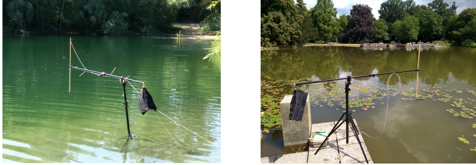
Figure 4.4: Measurement setup of the RoX spectrometer at a natural water body (left) and artificial ponds (right). Taken from [23]
