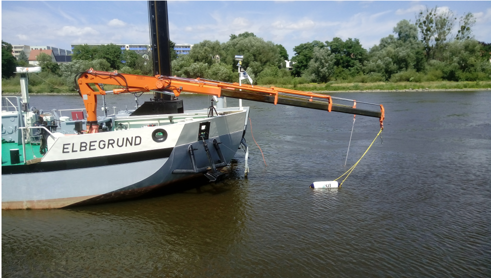
Figure 4.2: Application of the three sensor systems on the research vessel Elbegrund . The cranes on the front carries the Biofish sensor system (white floating cylinder, front right) and the PhycoSens collects water (front left) in the river Elbe. The hyperspectral sensor is mounted close to the railing in between the cranes. Taken from [22].
