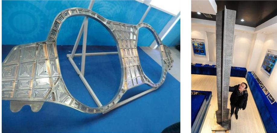
Figure 2: Selective laser sintering (SLS) for 3D printing of large scale objects made of titanium alloys for application in aircraft industry (a) C919 aircraft cockpit window frame [16], (b) 5 m high wing carrier [14].
