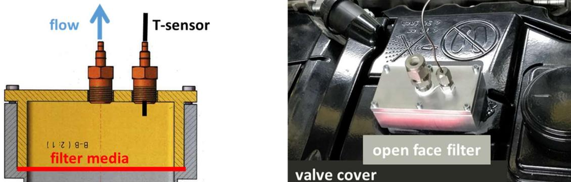
**Figure 3-24:** A schematic representation of the open face filter (left) and a photograph of the filter installed in the valve cover of the Daimler OM 934 engine (right).
