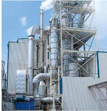
Figure 1.1: One-Effect FFE with MVR to concentrate wheat starch effluent
