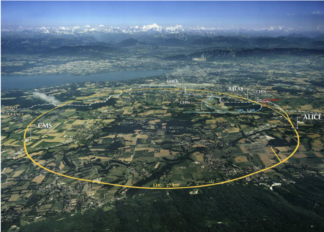
Figure 2.2: The location of the LHC around the CERN site nearby Geneva is shown as an overlay of an aerial view of the region. The large experiments ATLAS and CMS are located at opposite points on the ring while the smaller experiments ALICE and LHCb are located closer to the main site in caverns built for LEP. Credit: CERN, from [All13]
