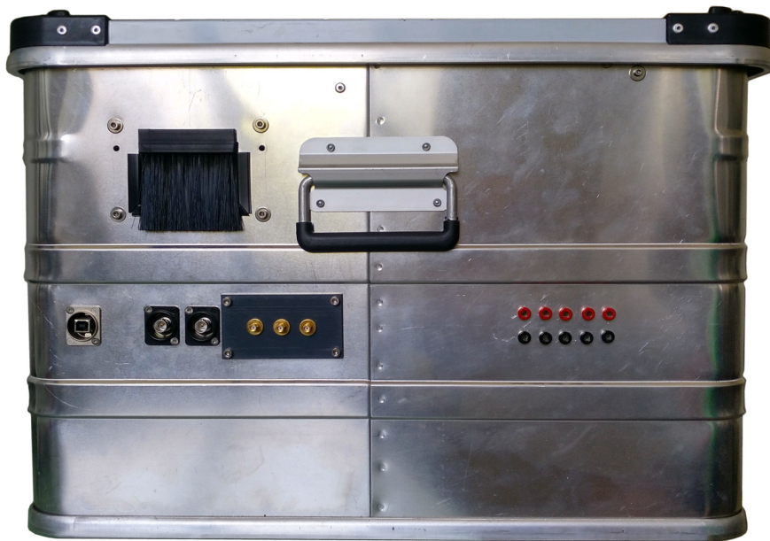
Figure 4.13: The ten flanges for laboratory measurement lines, the three SMA flanges and the two BNC flanges (right to left) enable the operation of the DUT setup inside the box mostly without cables fed through the light trap at the top. The USB flange is used for both the DUT system and the laser setup itself via an USB hub inside the box.
