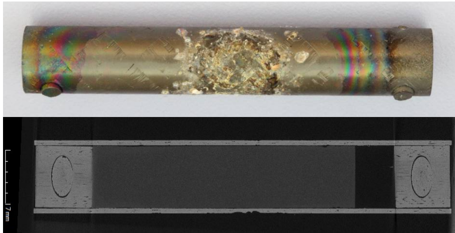
Fig. 4: Post-test appearance of the sample after the transient test up to 1845°C (top) and X-ray tomography longitudinal cut (bottom)
