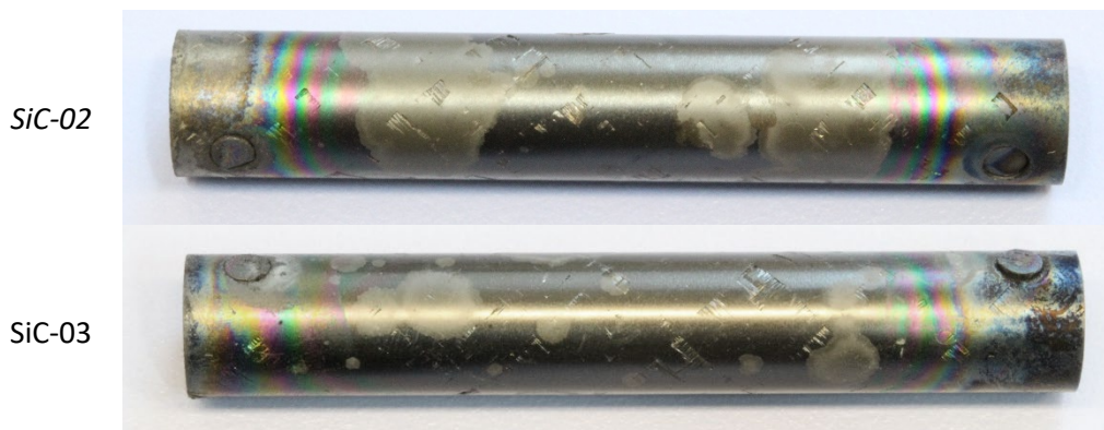
Fig. 7: Post-test appearance of the samples after 1 h isothermal oxidation in steam at 1700°C
