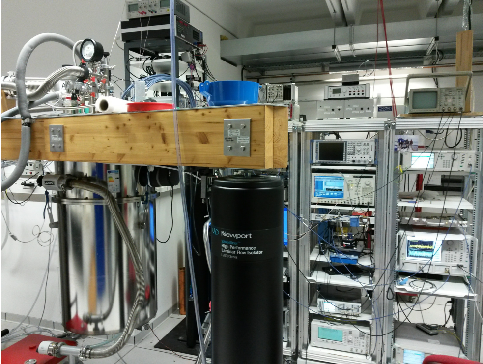
Figure 2.11: Photograph of a typical measurement setup for superconducting circuits. On the left, a closed-cycle dilution refrigerator is visible. Above it, multiple voltage supplies as well as room temperature amplifiers can be spotted. On the right, multiple racks with laboratory equipment are visible. These include RF frontend electronics as well as AWGs and current sources, but also more generic measurement equipment like vector network analyzers (VNAs) or spectrum analyzers. The picture was taken in 2017 inside the laboratory of the Institute of Physics (PHI) at the Karlsruhe Institute of Technology (KIT).
