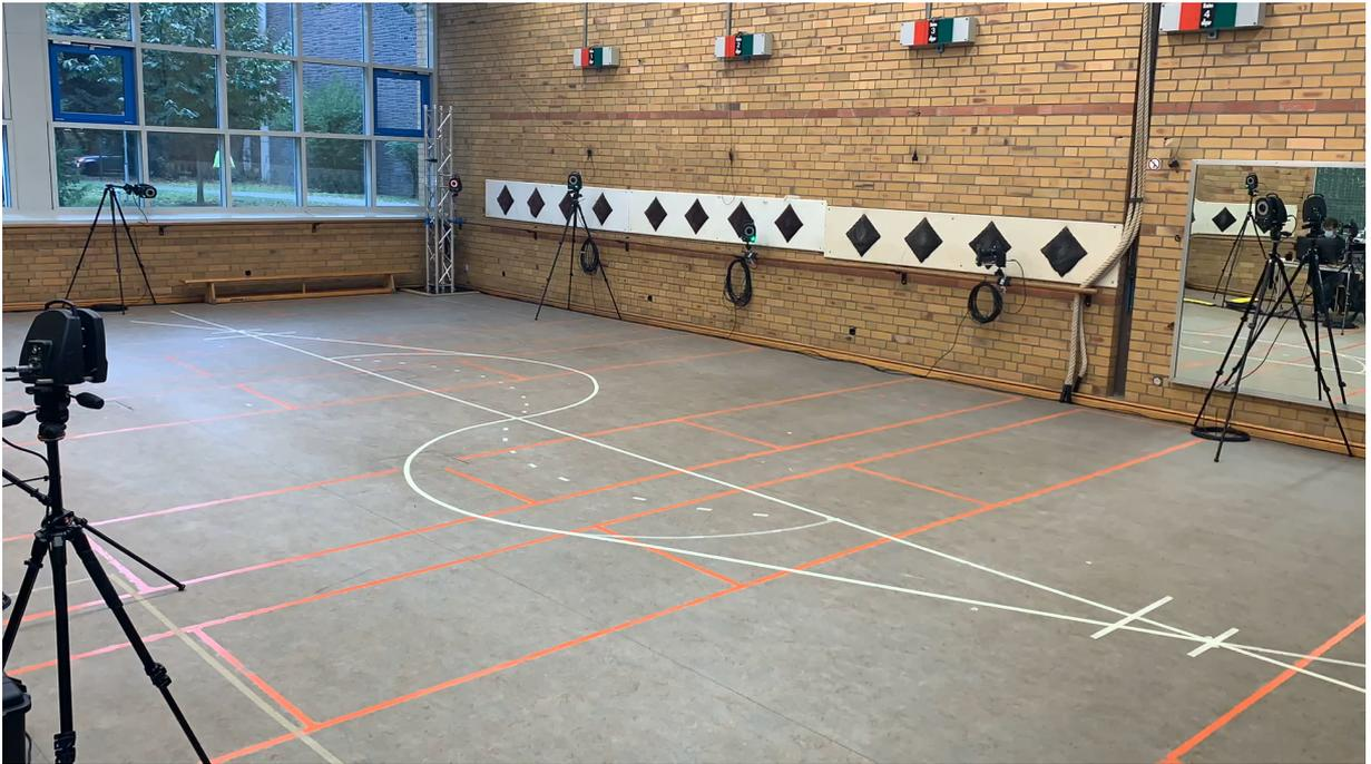
**Figure 7.5.:** Evaluation environment at German Sport University Cologne in the project Learning Robotic-Assistance Systems for Neuro-Muscular Training. The two paths, “line” and “curve”, are marked with white tape. In the right lower corner, cross lines mark the starting position for the line. Author: Björn Braunstein, October 16, 2020
