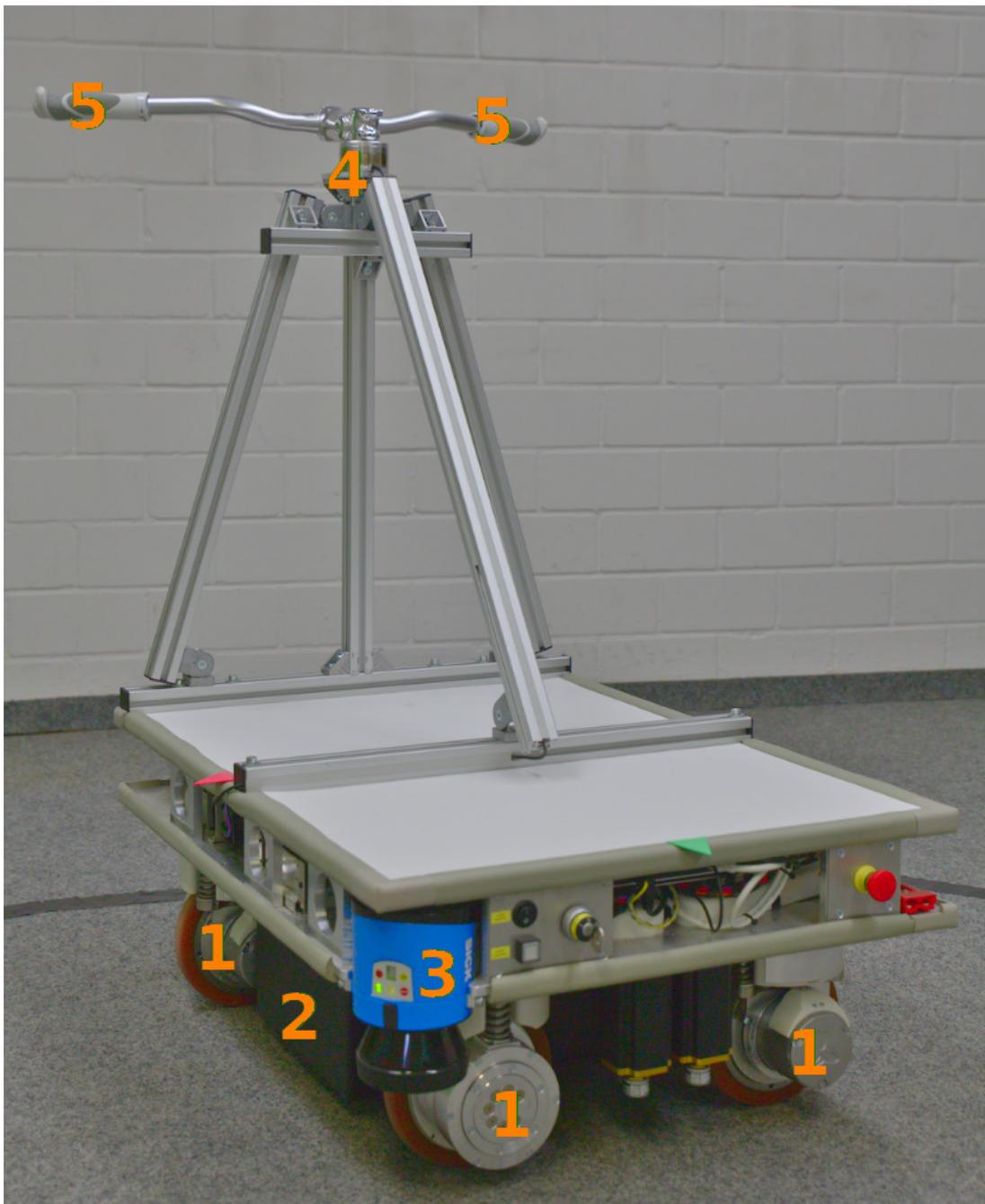
**Figure 3.2.:** The RoboTrainer Prototype as used in the HEiKA pilot study. Its main components are independently controllable drive-steer modules (1), a rechargeable battery pack (2), SICK LMS100 laser range scanners (3), a force-torque sensor (4), and a bike handlebar for controlling the robotic device (5).
