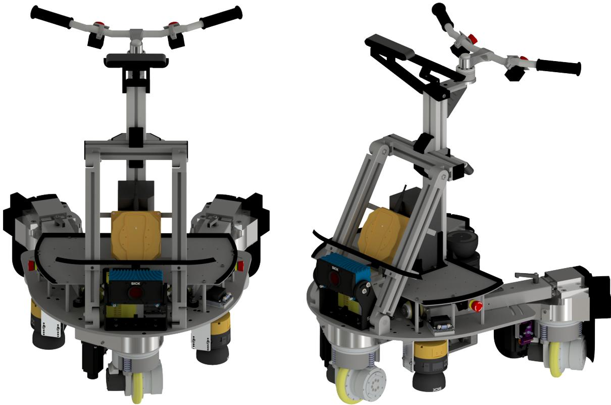
**Figure 4.2.:** RoboTrainer v2 CAD model (front view - left; side view - right).
