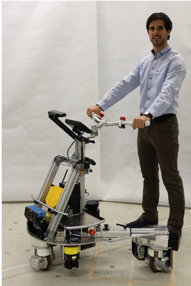
**Figure 4.1.:** RoboTrainer v2 and its user on the test parkour at the Institute for Anthropomatics and Robotics - Intelligent Process Control and Robotics. The markings on the floor represent paths and RoboTrainer’s positions which a user has to follow.
