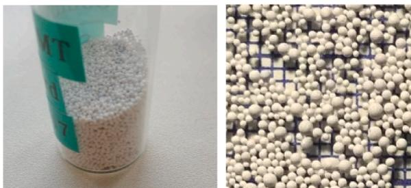
Fig. 1. Samples of two-phase lithium ceramic in the form of pebbles.
