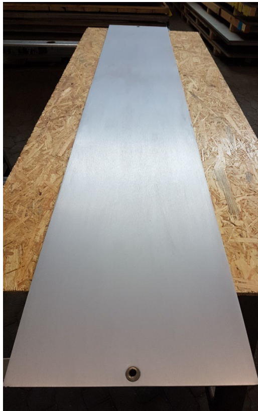
Zr sheet (thickness 3 mm) PVD coated with Cr (10 \mu\text{m} , X-ray measured) at one side
