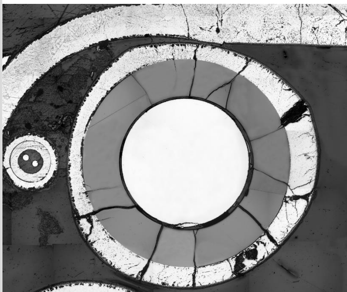
peripheral rod #13: melt between outer \alpha -Zr(O) and pellet
