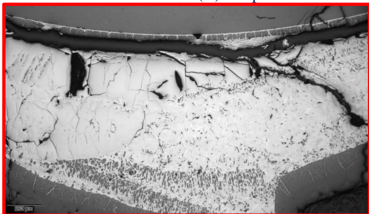
internal rod #4: melt (relocated from above) between outer \alpha -Zr(O) and pellet
