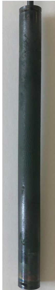
MC-5: 1200 °C during 15 min
