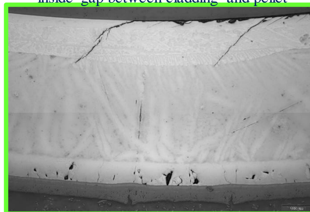
peripheral rod #12: melt relocated from above inside gap between cladding and pellet
