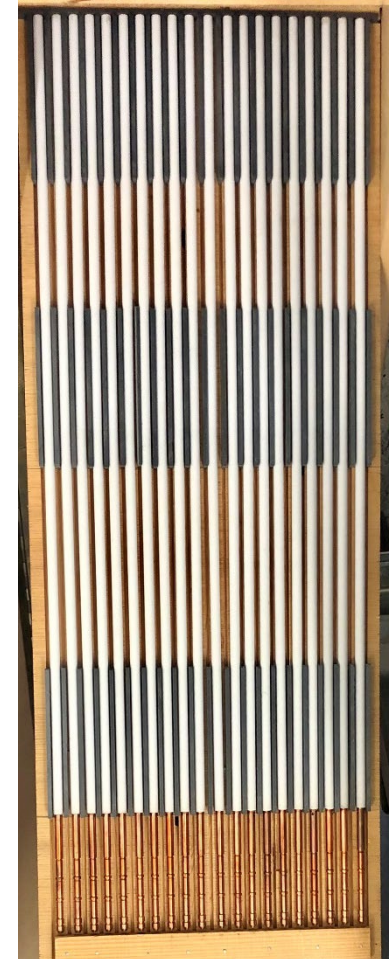
24 Mo/Cu lower electrodes partially coated by ZrO 2 (200 μm) OD 7.75 mm in coated region
