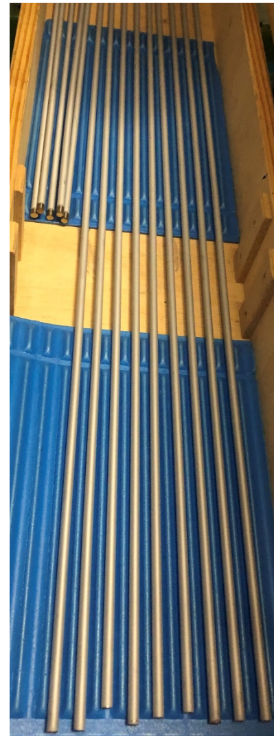
corner rods and tubes (OD 6 mm) PVD coated with Cr (10 µm)
