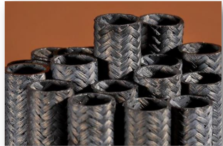
SiC-SiC cladding tubes
