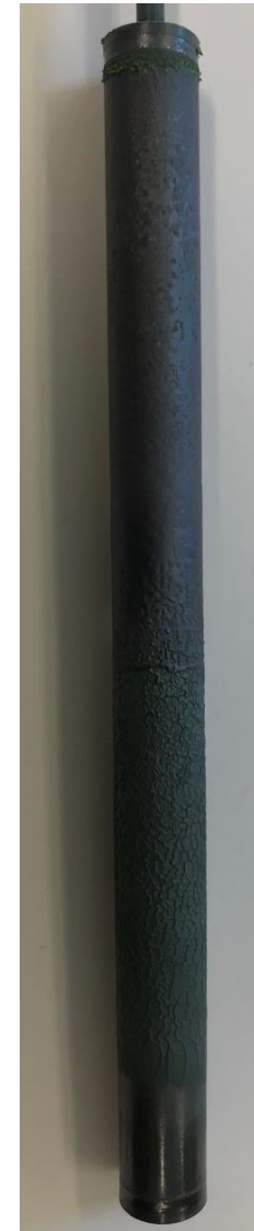
MC-6: 1350 °C during 5 min
