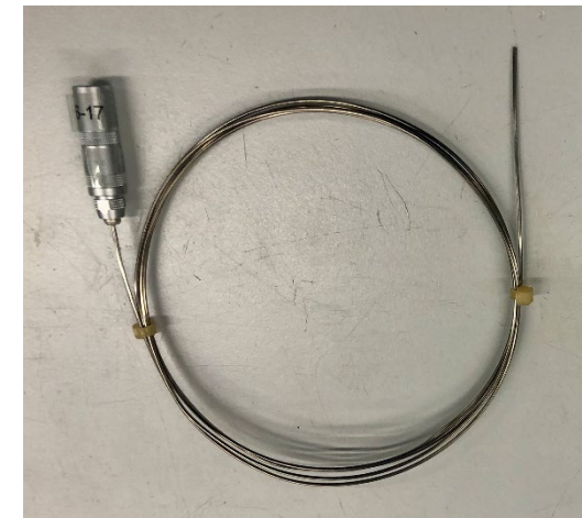
75 NiCr/Ni thermocouples sheathed with stainless steel
