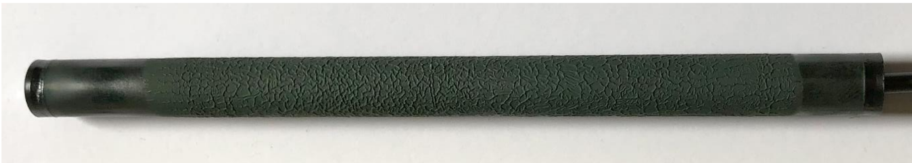
sample MCs-2: transient with 8 K/s, then 1400 °C during 240 s
