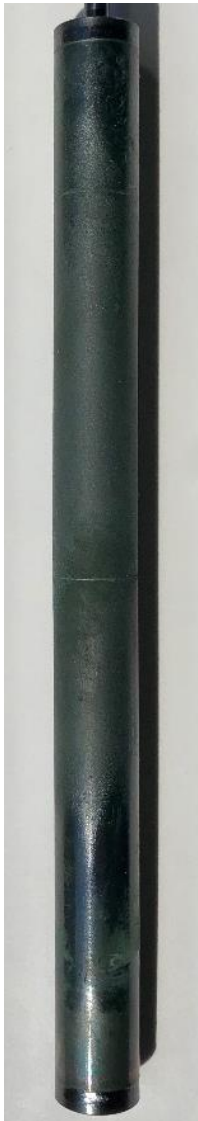
MC-4: 1200 °C during 10 min
