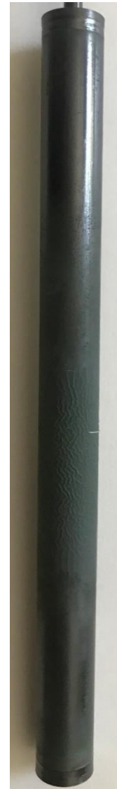
MC-7: 1250 °C during 10 min
