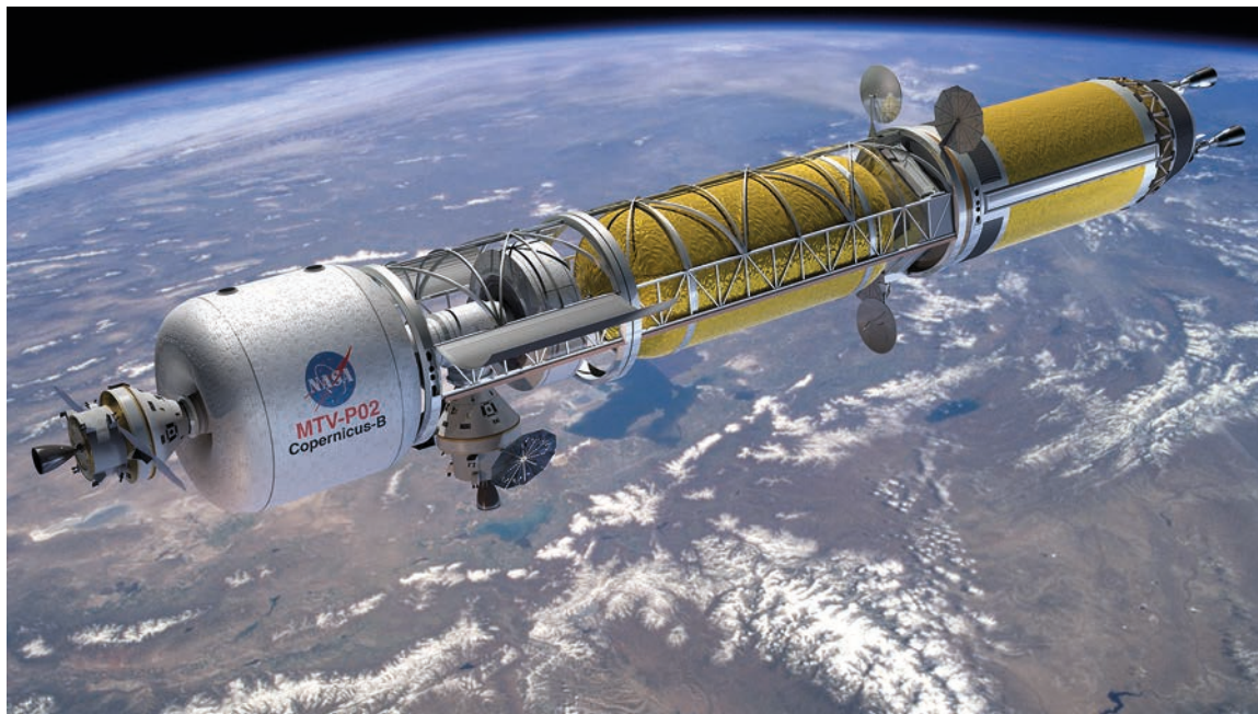
Fig.7 A Mars Transfer Vehicle of the Mars Design Reference Mission 5.0 concept study of NASA. [18]
