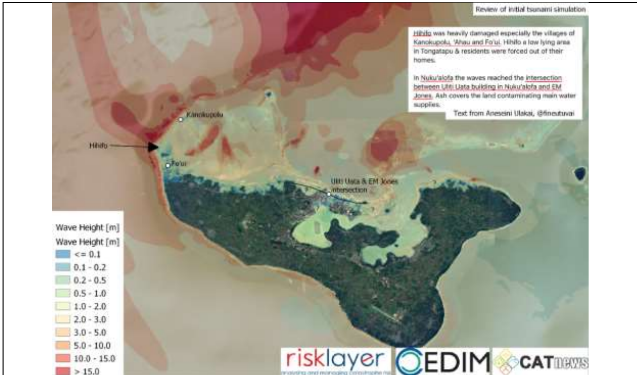
Comparison of initial tsunami inundation simulation with first local reports.
